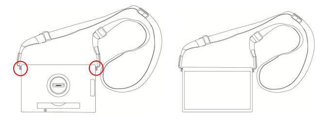
1. Align and attach the shoulder strap to the tablet as shown and fasten the screws (x2) to secure it.
