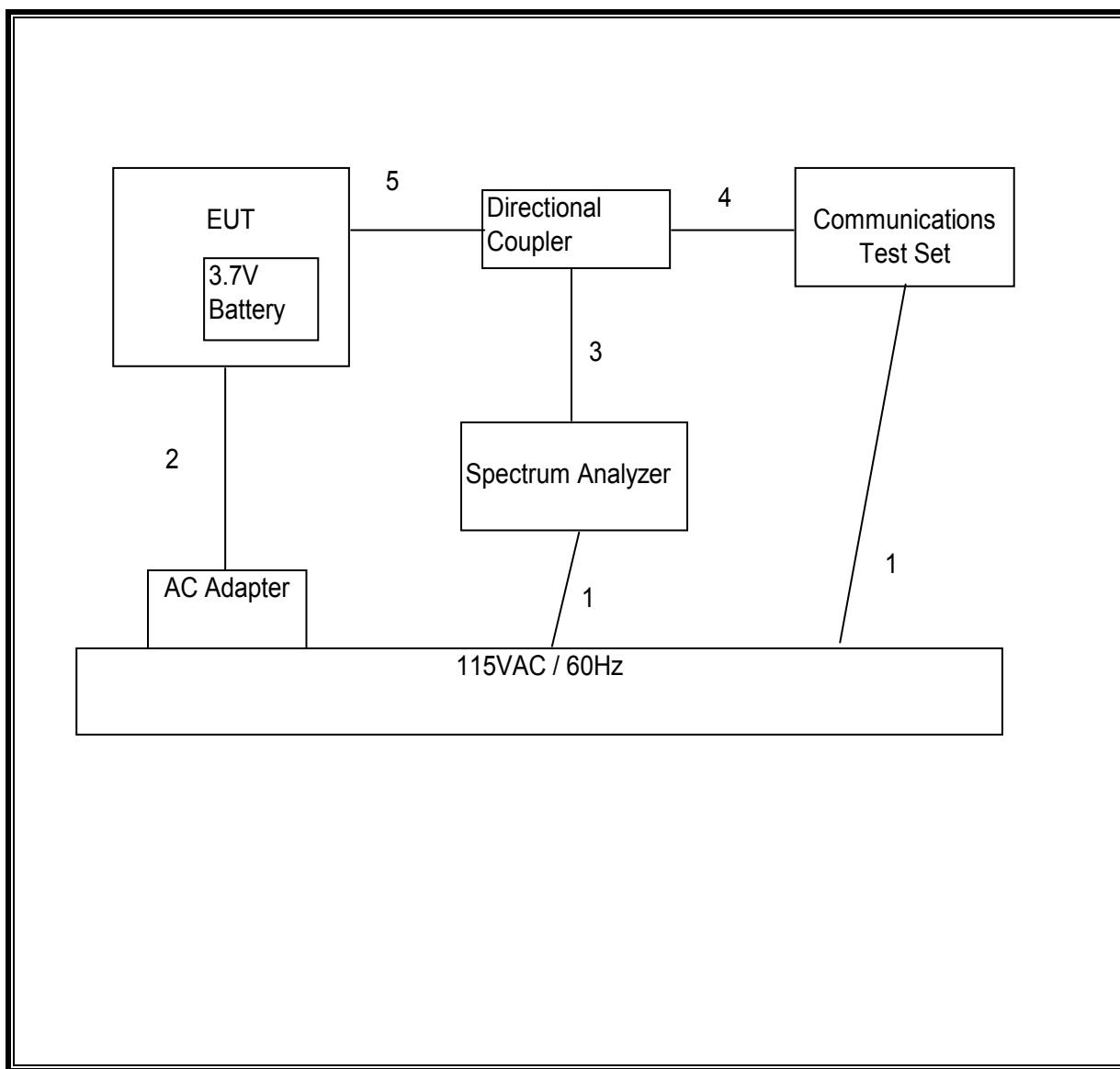
**SETUP DIAGRAM FOR RADIATED TESTS**
