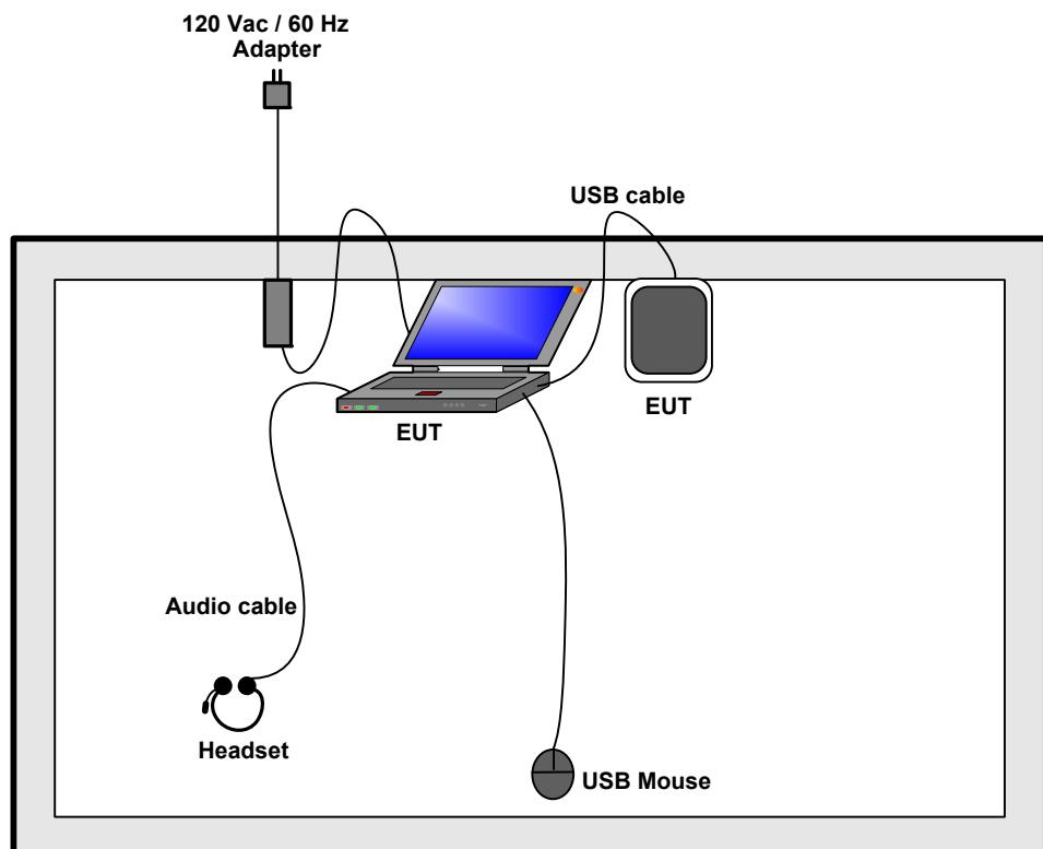
Test Setup Diagram – Radiated Test (Above 1GHz)
