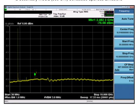
■ Secondary MODE (684 CH.) Conducted Spurious Emissions
