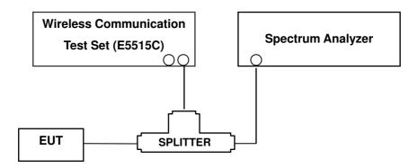
(Configuration of conducted Emission measurement)
