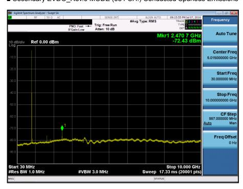
■ Secondary EVDO\_Rev.A MODE (476 CH.) Conducted Spurious Emissions
