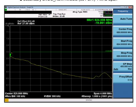
■ Secondary MODE (476 CH.) Conducted Spurious Emissions
