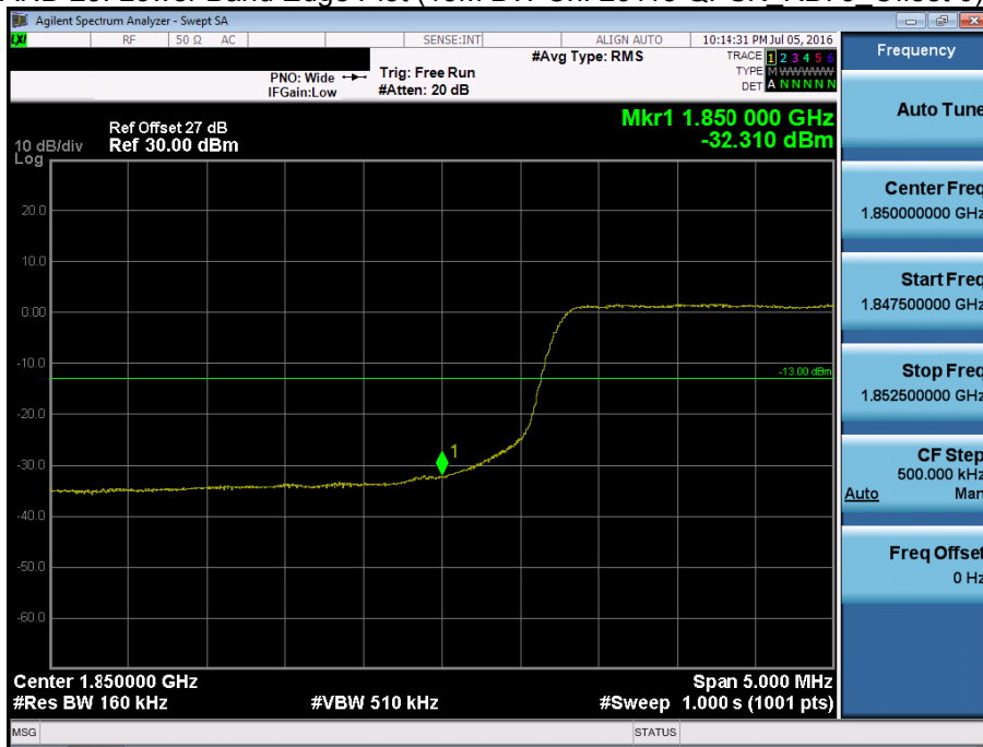
BAND 25. Lower Band Edge Plot (15M BW Ch. 26115 QPSK_RB75_Offset 0) -2
