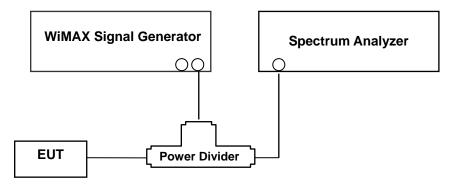
(Configuration of conducted Emission measurement) Test Procedure
