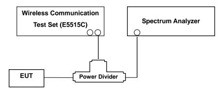
(Configuration of conducted Emission measurement) Test Procedure
