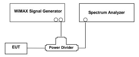
(Configuration of conducted Emission measurement) Test Procedure
