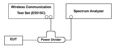
(Configuration of conducted Emission measurement) Test Procedure
