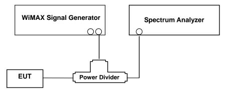
(Configuration of conducted Emission measurement) Test Procedure
