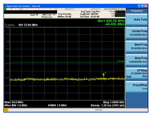
■ QPSK MODE 1/2 (2501.0 MHz) Conducted Spurious Emissions2
