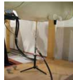
Photo of the dipole Antenna
