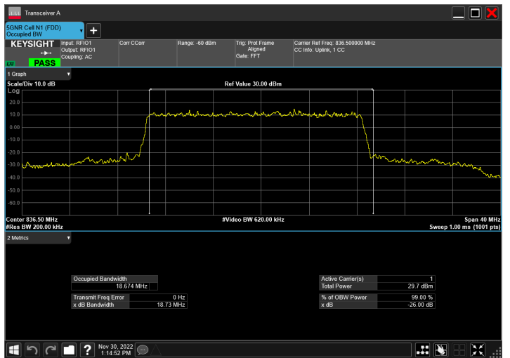
DC_2A_n5A_10MHz|20MHz_15kHz_1880MHz|836.5MHz_QP SK|DFT-s-OFDM 16 QAM_RB1@50|RB100@0
