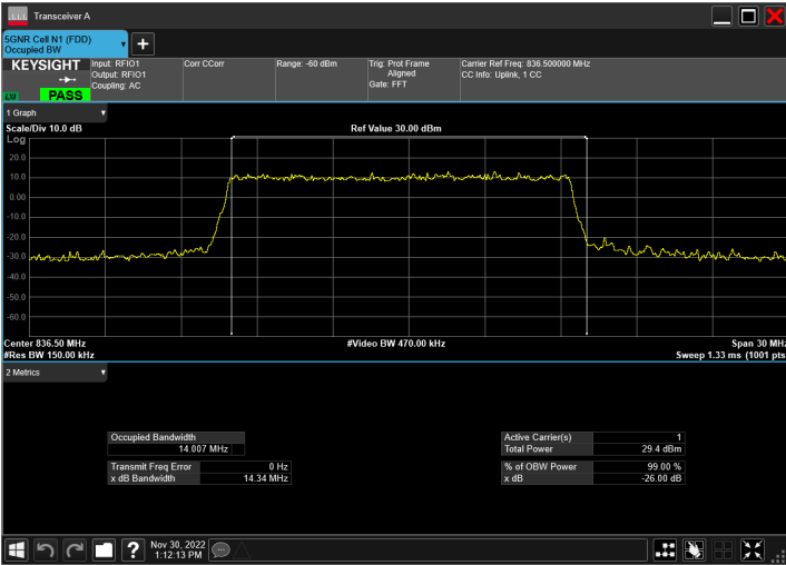
DC_2A_n5A_10MHz|15MHz_15kHz_1880MHz|836.5MHz_QP SK|CP-OFDM 16 QAM_RB1@50|RB79@0
