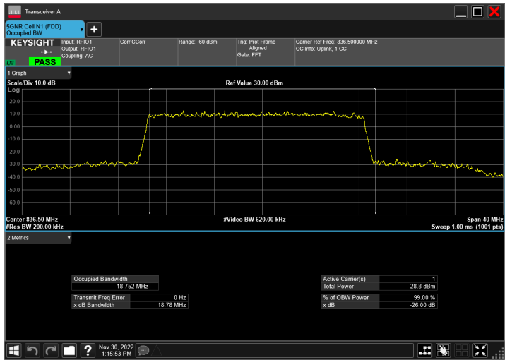
DC_2A_n5A_10MHz|20MHz_15kHz_1880MHz|836.5MHz_QP SK|CP-OFDM 16 QAM_RB1@50|RB106@0
