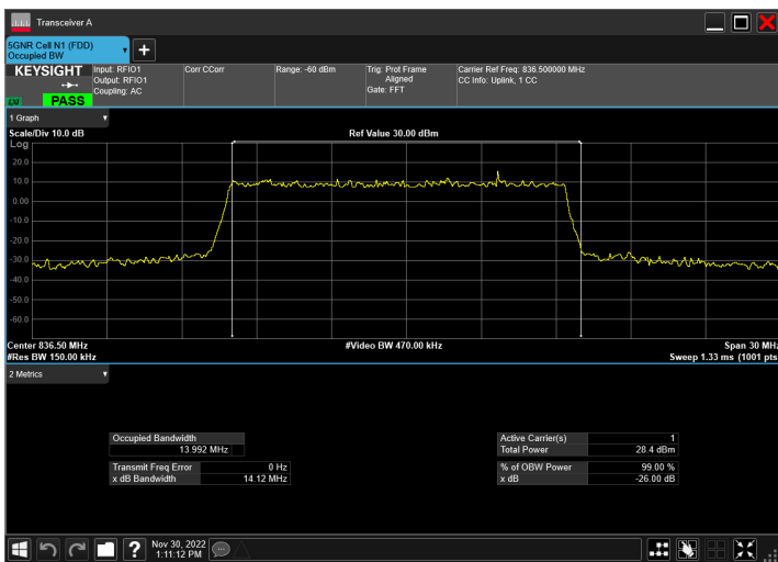
DC_2A_n5A_10MHz|15MHz_15kHz_1880MHz|836.5MHz_QP SK|DFT-s-OFDM 256 QAM_RB1@50|RB75@0
