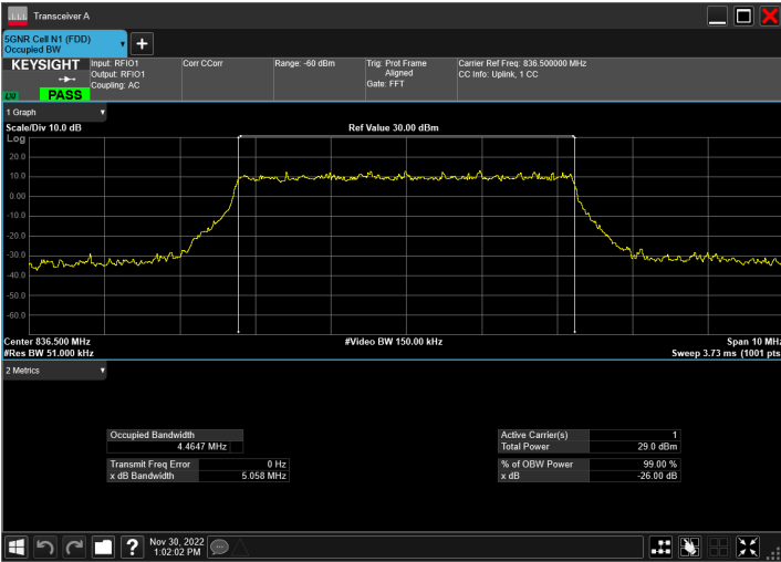
DC_2A_n5A_10MHz|5MHz_15kHz_1880MHz|836.5MHz_QPS K|CP-OFDM 16 QAM_RB1@50|RB25@0
