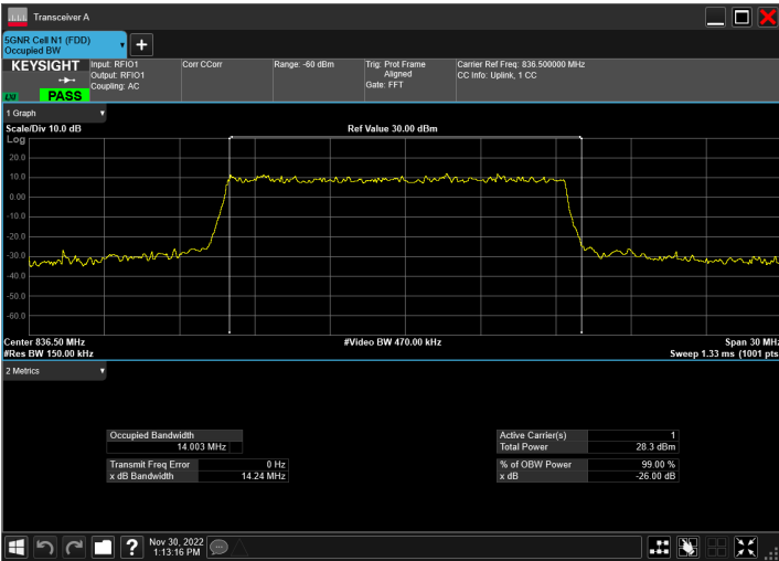
DC_2A_n5A_10MHz|15MHz_15kHz_1880MHz|836.5MHz_QP SK|CP-OFDM 256 QAM_RB1@50|RB79@0
