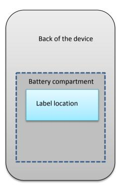
The label is placed in the battery compartment and it is viewable for the users as they install the SIM card.
