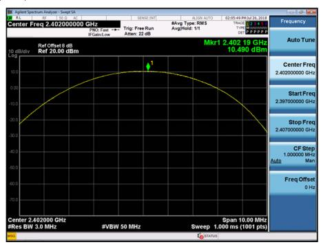
Test Plots (π/4DQPSK) Peak Power (CH.39)
