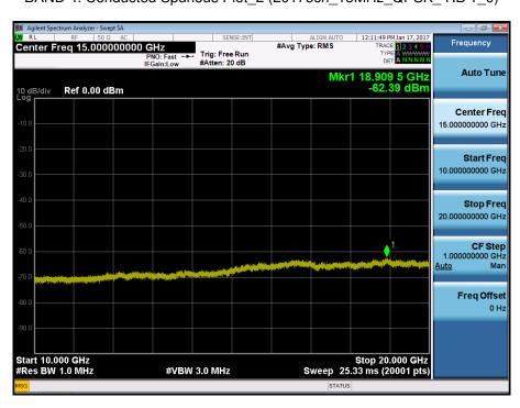
BAND 4. Conducted Spurious Plot\_1 (20325ch\_15MHz\_QPSK\_ RB 1\_0)
