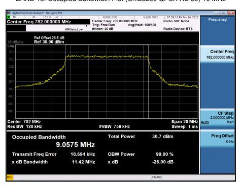
BAND 13. Occupied Bandwidth Plot (Ch.23230 16-QAM RB 50) 10 MHz
