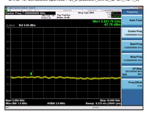
BAND 13. Conducted Spurious Plot\_1 (23230ch\_5MHz\_QPSK\_RB 1\_0)
