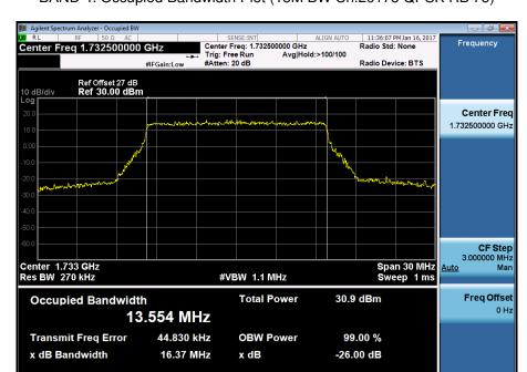
BAND 4. Occupied Bandwidth Plot (15M BW Ch.20175 16QAM RB 75)
