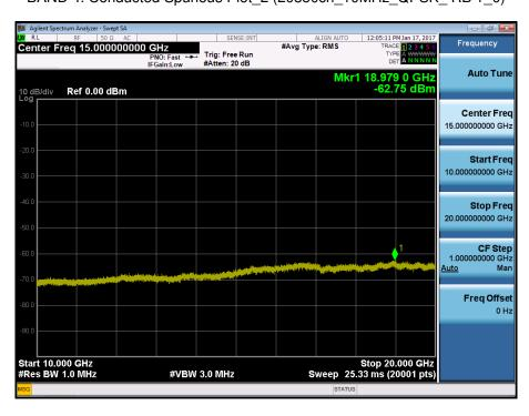
BAND 4. Conducted Spurious Plot\_1 (20025ch\_15MHz\_QPSK\_ RB 1\_0)
