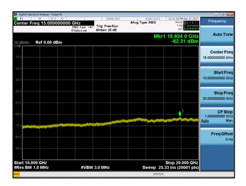
BAND 4. Conducted Spurious Plot\_1 (20175ch\_15MHz\_QPSK\_ RB 1\_0)
