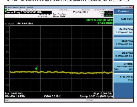
BAND 13. Conducted Spurious Plot 1 (Ch.23230 10 MHz QPSK RB 1, Offset 0)
