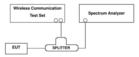
(Configuration of conducted Emission measurement)
