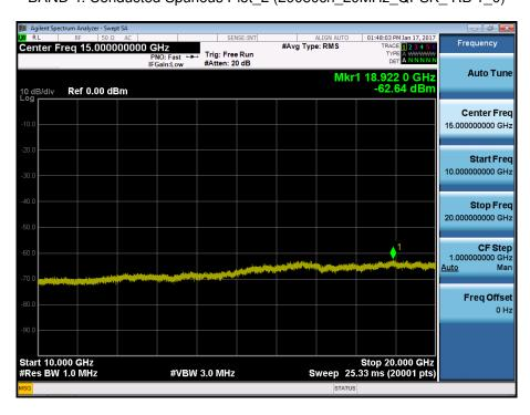
BAND 4. Conducted Spurious Plot\_1 (20175ch\_20MHz\_QPSK\_ RB 1\_0)
