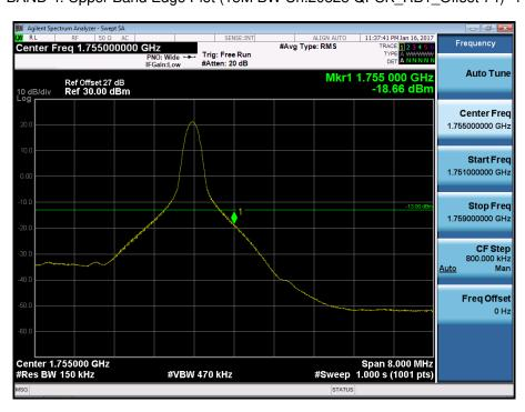
BAND 4. Upper Band Edge Plot (15M BW Ch.20325 QPSK\_RB75) -2
