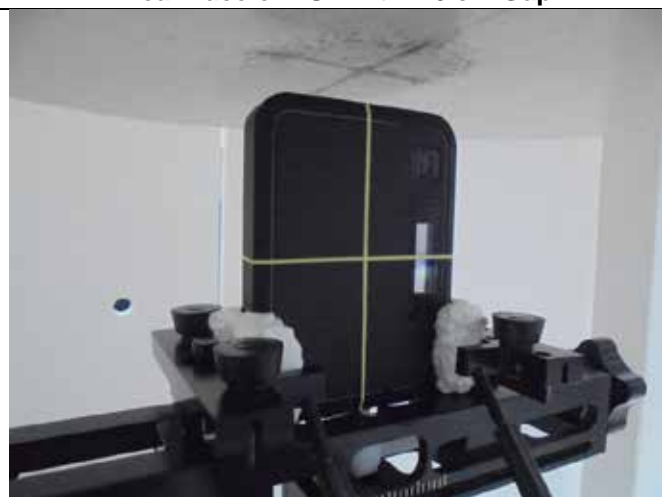
Right Side of EUT with 1.0 cm Gap
