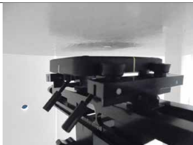
Rear Face of EUT with 1.0 cm Gap
