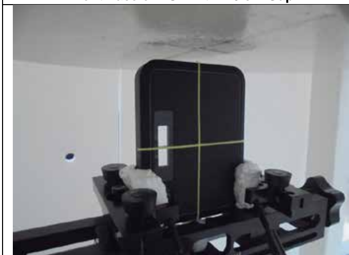
Left Side of EUT with 1.0 cm Gap
