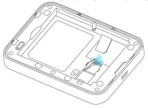
5. Remove the SIM card by gently pressing down and sliding outwards.
