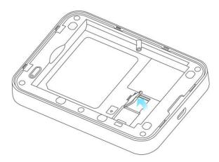
4. Insert the SIM card gently with gold IC chip facing downward
