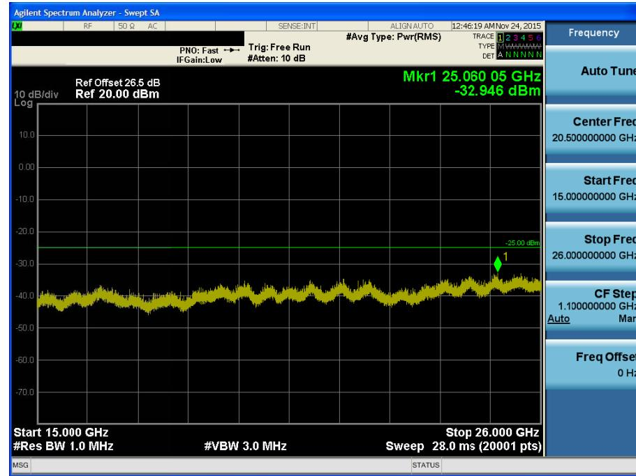
BAND 41. Conducted Spurious Plot 1 (15 MHz Ch.41515 QPSK RB 1, Offset 0)
