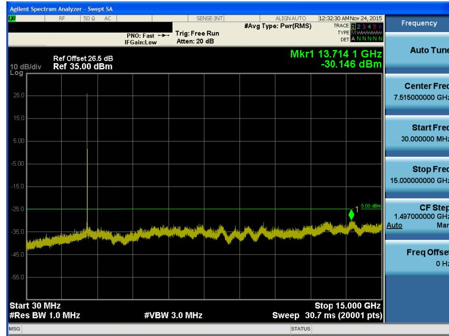
BAND 41. Conducted Spurious Plot 2 (15 MHz Ch. 40620 QPSK RB 1, Offset 0)
