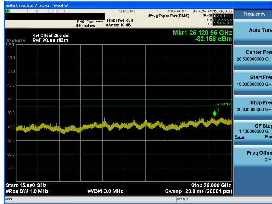
BAND 41. Conducted Spurious Plot 1 (20 MHz Ch.41490 QPSK RB 1, Offset 0)
