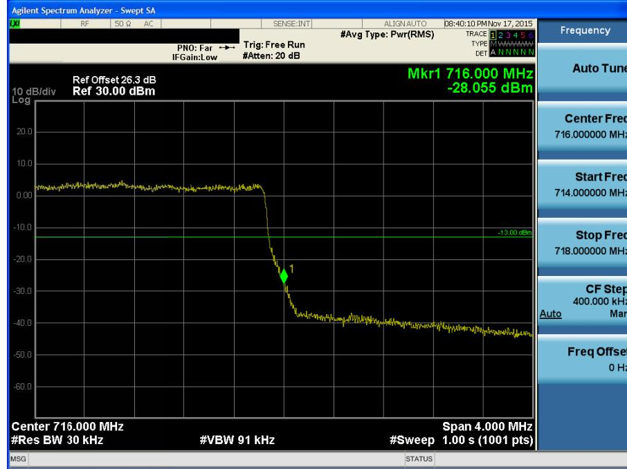
BAND 12. Upper Extended Band Edge Plot (3M BW Ch.23165 QPSK\_RB15\_0)
