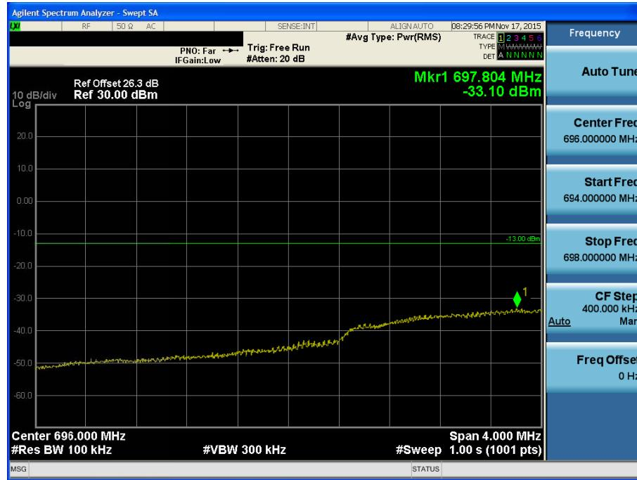
BAND 12. Lower Band Edge Plot (5M BW Ch.23035 QPSK\_RB1\_Offset 0)
