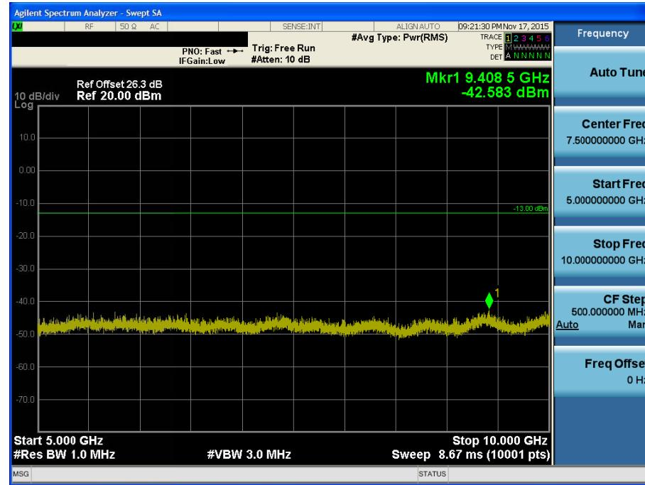
BAND 12. Conducted Spurious Plot \_1 (23095ch\_3MHz\_QPSK\_RB 1\_0)
