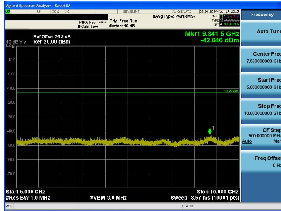
BAND 12. Conducted Spurious Plot \_1 (23060ch\_10MHz\_QPSK\_RB 1\_0)
