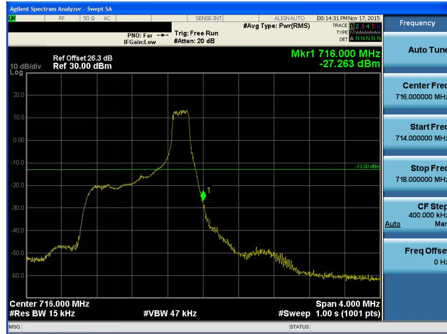
BAND 12. Upper Band Edge Plot (1.4M BW Ch.23173 QPSK\_RB6\_Offset 0)
