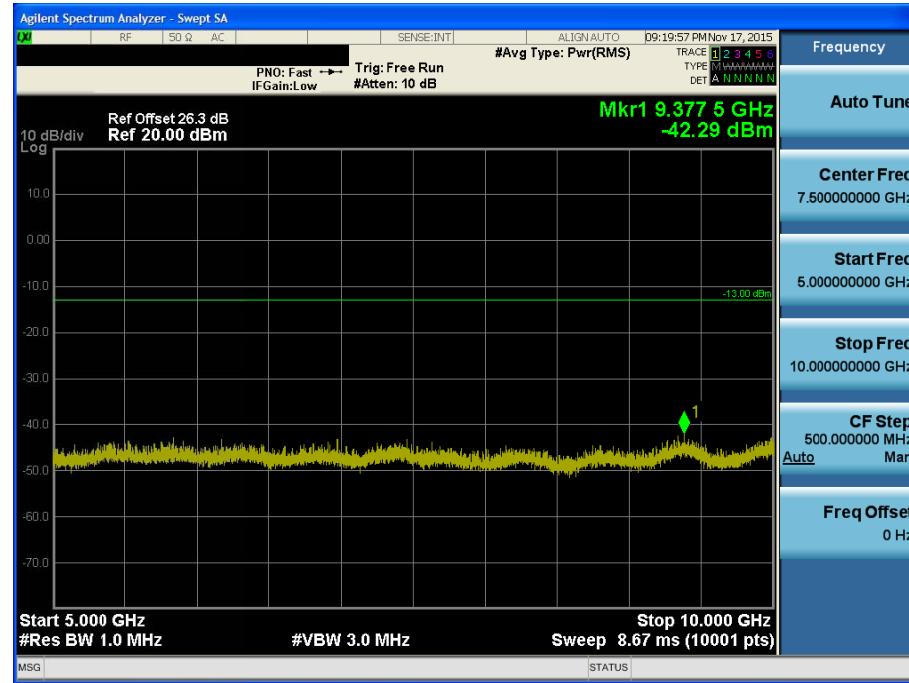
BAND 12. Conducted Spurious Plot \_1 (23173ch\_1.4MHz\_QPSK\_RB 1\_0)
