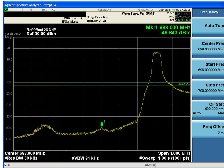
BAND 12. Lower Band Edge Plot (3M BW Ch.23025 QPSK\_RB15\_Offset 0)
