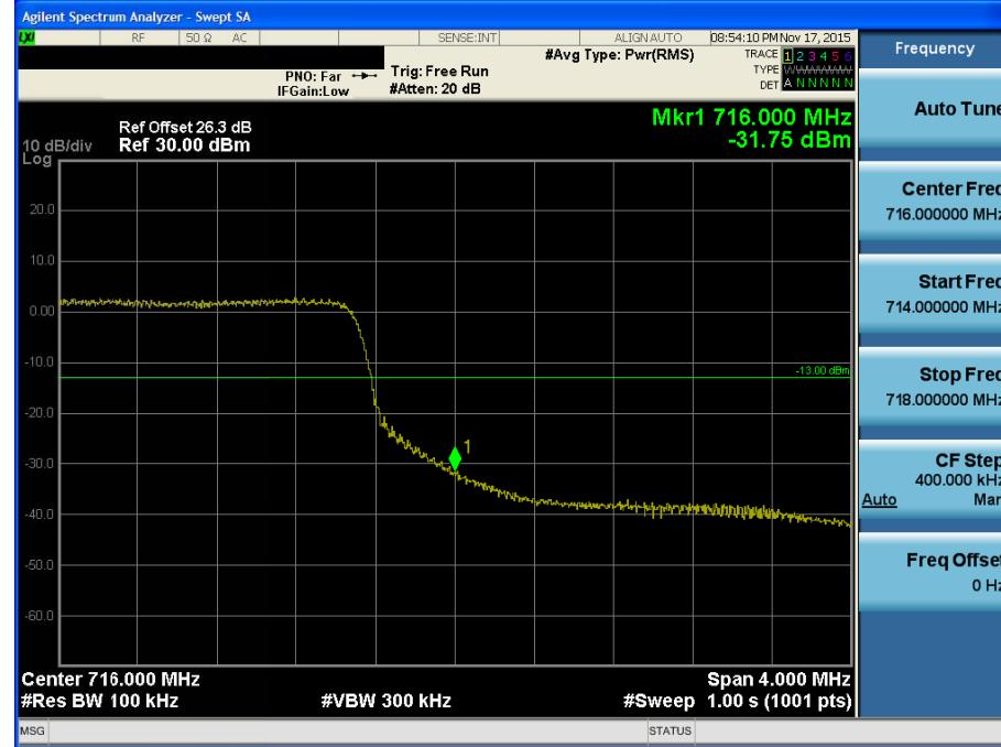
BAND 12. Upper Extended Band Edge Plot (10M BW Ch.23130 QPSK\_RB50\_0)
