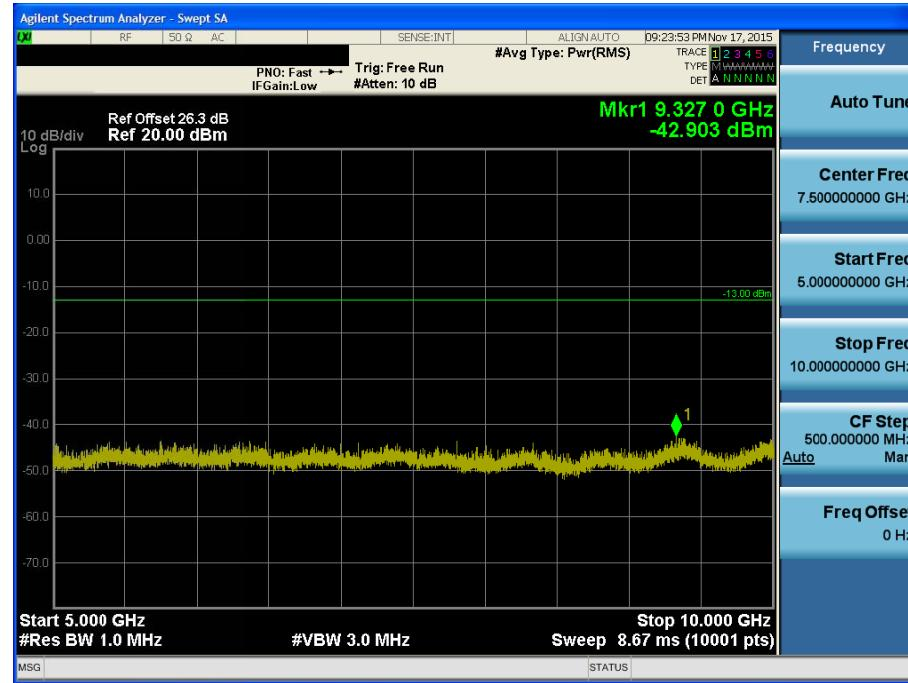
BAND 12. Conducted Spurious Plot \_1 (23155ch\_5MHz\_QPSK\_RB 1\_0)
