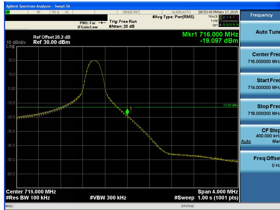
BAND 12. Upper Band Edge Plot (10M BW Ch.23130 QPSK\_RB50\_Offset 0)
