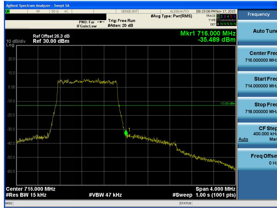
BAND 12. Upper Extended Band Edge Plot (1.4M BW Ch.23173 QPSK\_RB6\_0)
