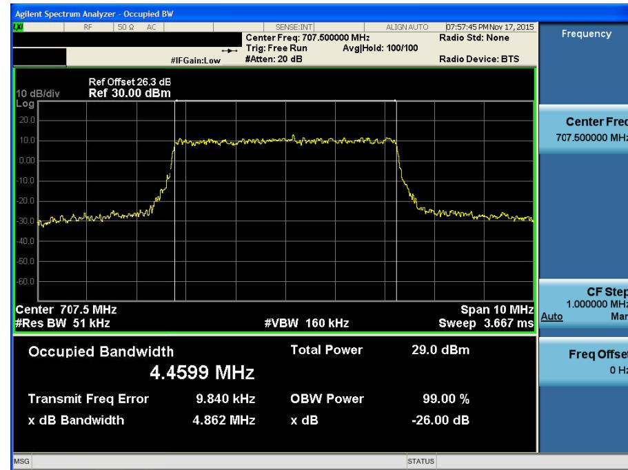
BAND 12. Occupied Bandwidth Plot (10M BW Ch.23095 QPSK\_RB50\_0)
