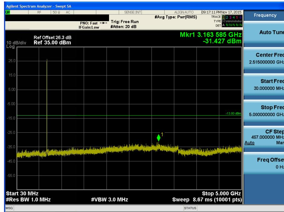
BAND 12. Conducted Spurious Plot \_2 (23017ch\_1.4MHz\_QPSK\_RB 1\_0)
