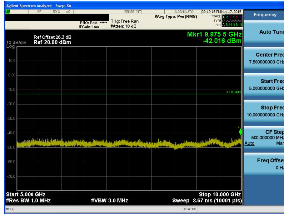
BAND 12. Conducted Spurious Plot \_1 (23025ch\_3MHz\_QPSK\_RB 1\_0)
