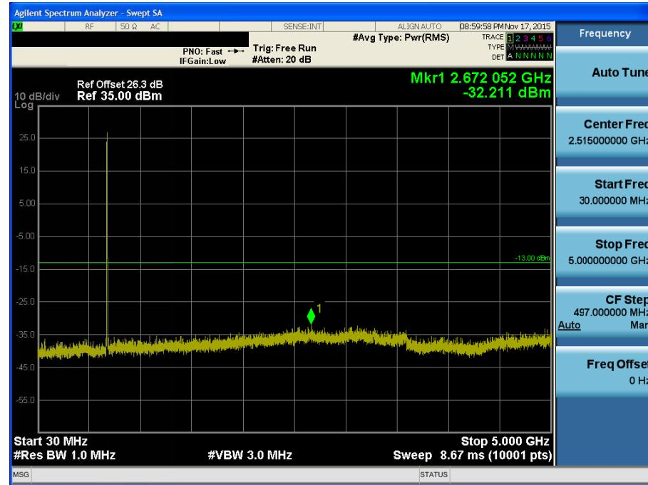
BAND 12. Conducted Spurious Plot \_2 (23035ch\_5MHz\_QPSK\_RB 1\_0)
