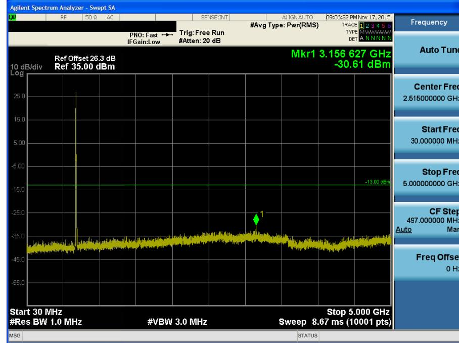
BAND 12. Conducted Spurious Plot \_2 (23060ch\_10MHz\_QPSK\_RB 1\_0)
