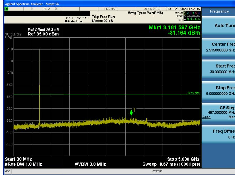
BAND 12. Conducted Spurious Plot \_2 (23173ch\_1.4MHz\_QPSK\_RB 1\_0)
