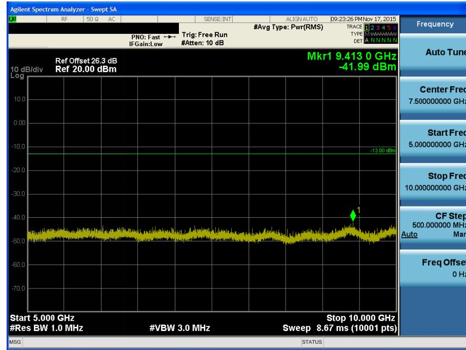
BAND 12. Conducted Spurious Plot \_1 (23095ch\_5MHz\_QPSK\_RB 1\_0)
