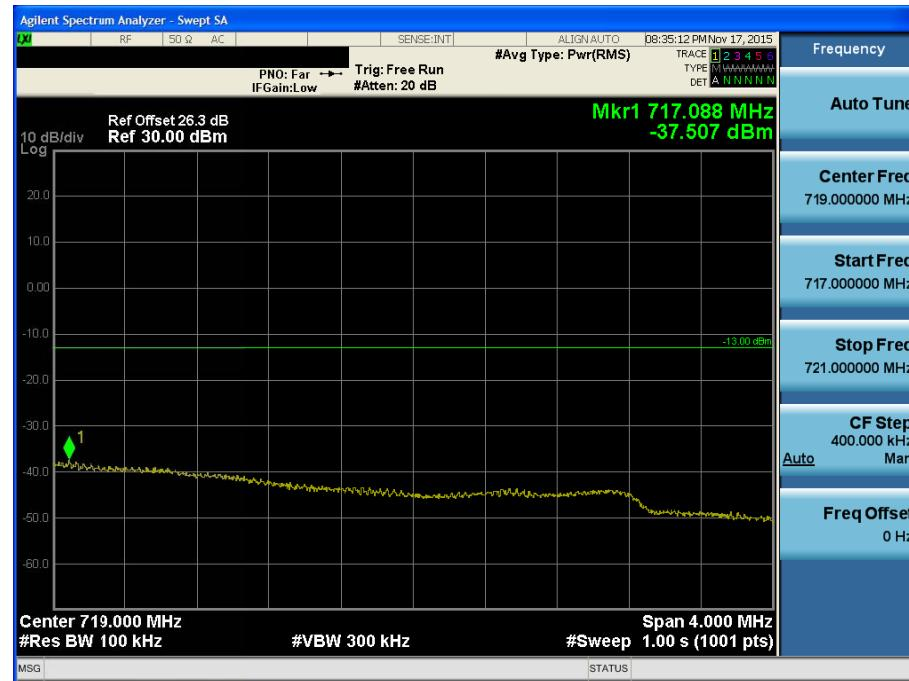
BAND 12. Upper Band Edge Plot (10M BW Ch.23130 QPSK\_RB1\_Offset 49)
