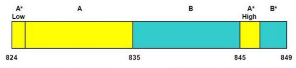
BLOCK 1: 824 – 835 MHz (A\* Low + A) BLOCK 2: 835 – 845 MHz (B) BLOCK 3: 845 – 846.5 MHz (A\* High) BLOCK 4: 846.5 – 849 MHz (B\*)
