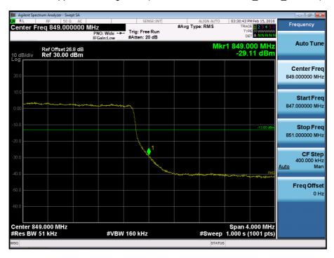
BAND 5. Upper Extended Band Edge Plot (5M BW Ch.20625 QPSK\_RB25\_0)
