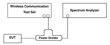
(Configuration of conducted Emission measurement)
