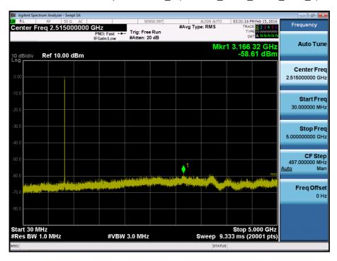
BAND 5. Conducted Spurious Plot \_2 (20625ch\_5MHz\_QPSK\_RB 1\_0)
