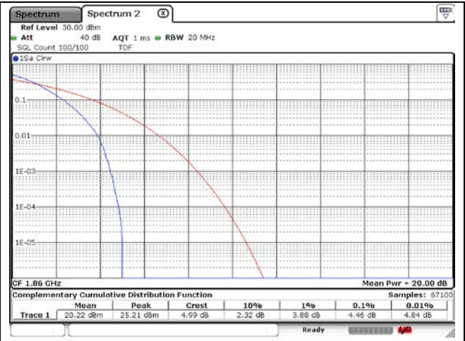
20 MHz QPSK Low Channel - Full RB
