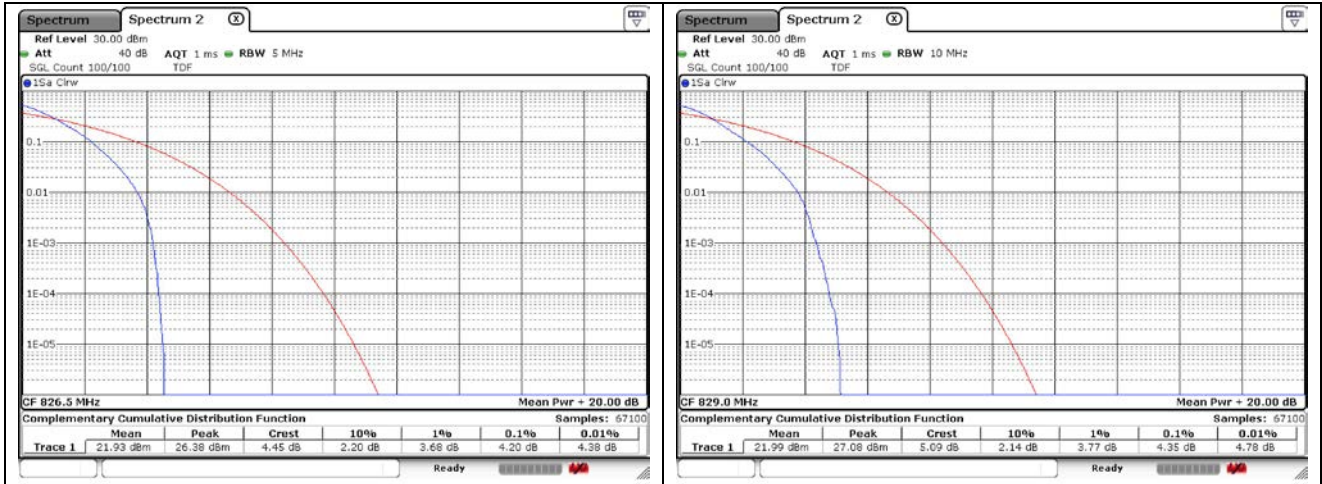
5 MHz QPSK Low Channel - Full RB
