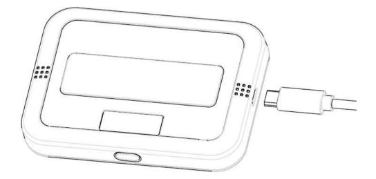
Unplug the AC adapter from the outlet, and remove the micro USB connector from the device.
