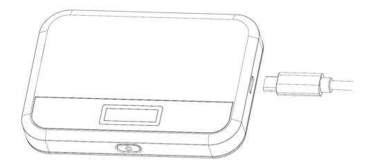
Unplug the AC adapter from the outlet, and remove the micro USB connector from the device.
