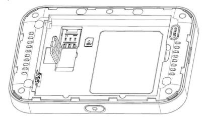
4. Insert the SIM card gently with gold IC chip facing downward
