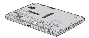
Put the battery back in place. Turn the computer over and reconnect the cables.
