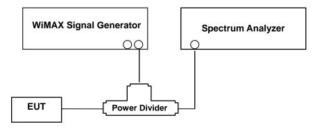
(Configuration of conducted Emission measurement) Test Procedure
