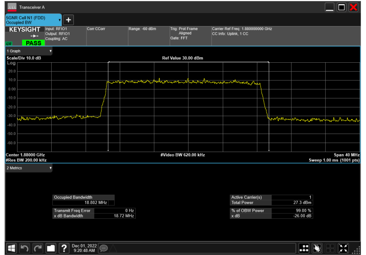
DC_66A_n2A_10MHz|20MHz_15kHz_1745MHz|1880MHz_Q PSK|DFT-s-OFDM 256 QAM_RB1@50|RB100@0
