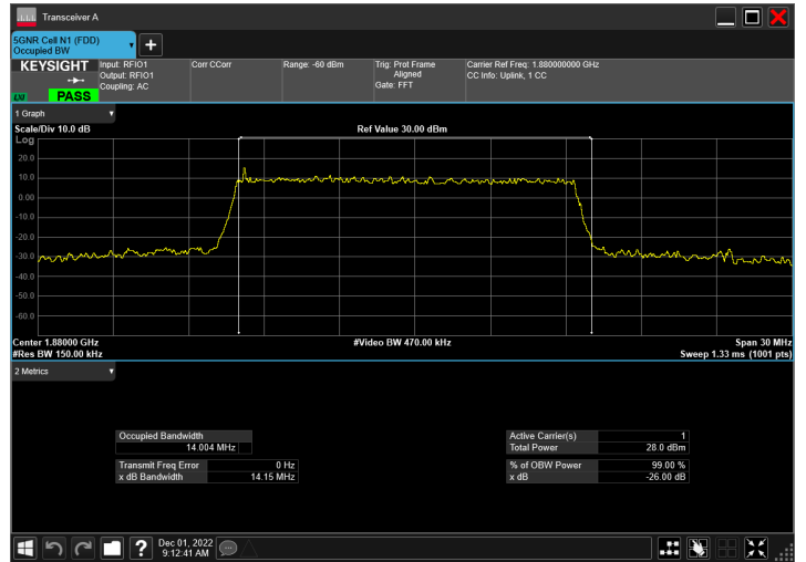
DC_66A_n2A_10MHz|15MHz_15kHz_1745MHz|1880MHz_Q PSK|DFT-s-OFDM 64 QAM_RB1@50|RB75@0
