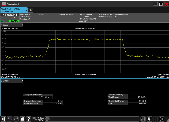
DC_5A_n2A_10MHz|15MHz_15kHz_836.5MHz|1880MHz_QP SK|CP-OFDM 256 QAM_RB1@50|RB79@0
