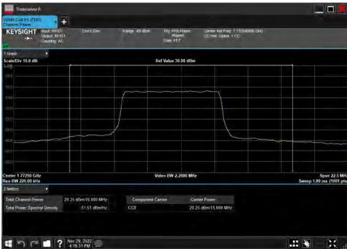
DC_2A_n66A_10MHz|15MHz_15kHz_1905MHz|1772.5MHz_ QPSK|DFT-s-OFDM 64 QAM_RB12@38|RB36@18
