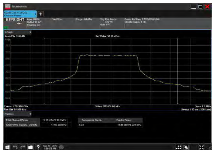
DC_5A_n66A_10MHz|5MHz_15kHz_829MHz|1712.5MHz_QP SK|DFT-s-OFDM 64 QAM_RB12@0|RB12@6
