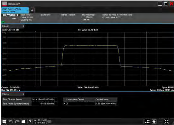
DC_2A_n66A_10MHz|30MHz_15kHz_1880MHz|1745MHz_Q PSK|CP-OFDM 16 QAM_RB12@0|RB80@40
