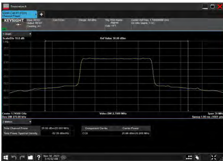
DC_5A_n66A_10MHz|20MHz_15kHz_836.5MHz|1745MHz_Q PSK|CP-OFDM 64 QAM_RB12@0|RB53@26
