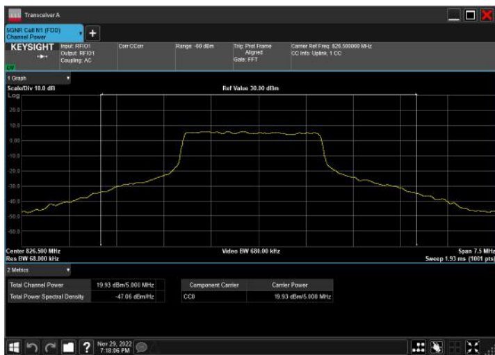
DC_2A_n5A_10MHz|5MHz_15kHz_1855MHz|826.5MHz_QPS K|DFT-s-OFDM QPSK_RB12@0|RB12@6
