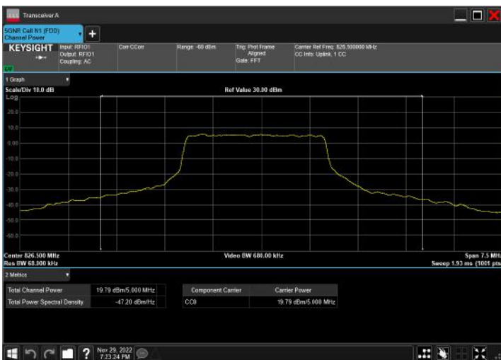
DC_2A_n5A_10MHz|5MHz_15kHz_1855MHz|826.5MHz_QPS K|CP-OFDM 64 QAM_RB12@0|RB13@6
