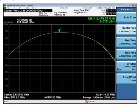
Test Plots (8DPSK) Peak Power (CH.0)
