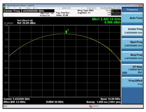
Test Plots (π/4DQPSK) Peak Power (CH.39)
