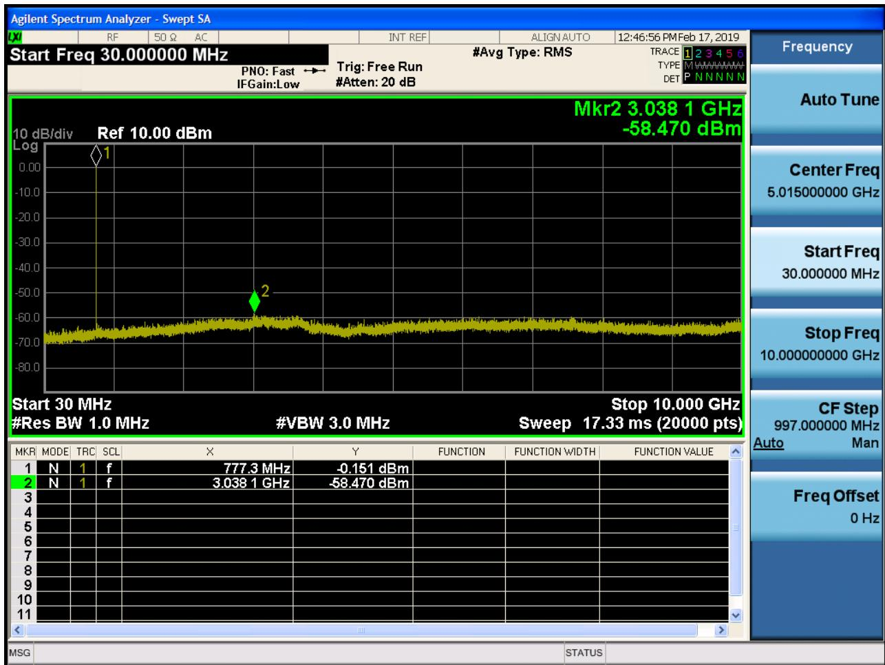
BAND 13. Conducted Spurious Plot (23230ch\_5MHz\_QPSK)
