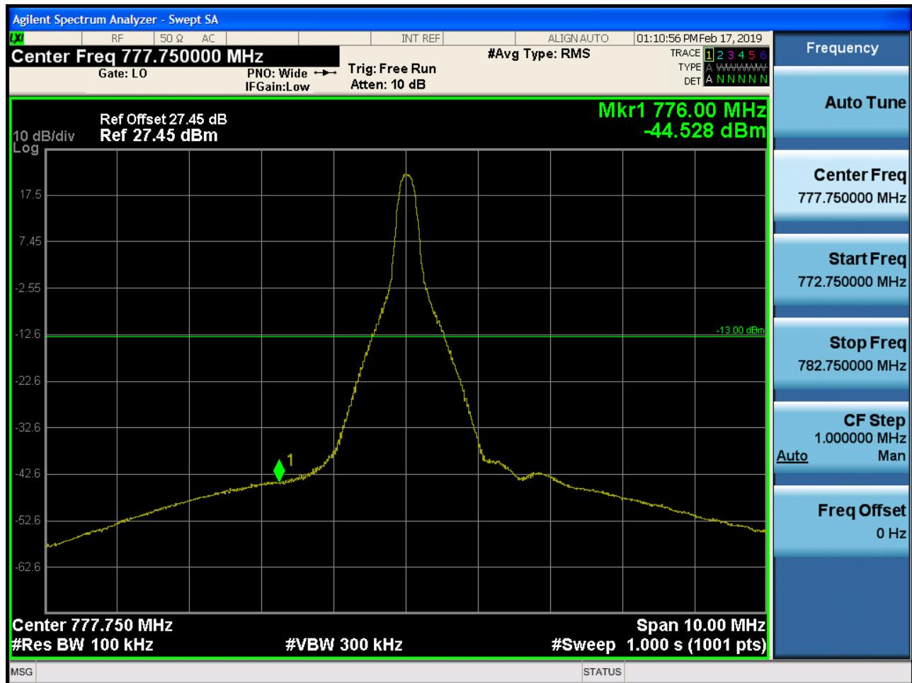
BAND 13. Lower Band Edge Plot (10M BW Ch.23230 QPSK\_Full RB)
