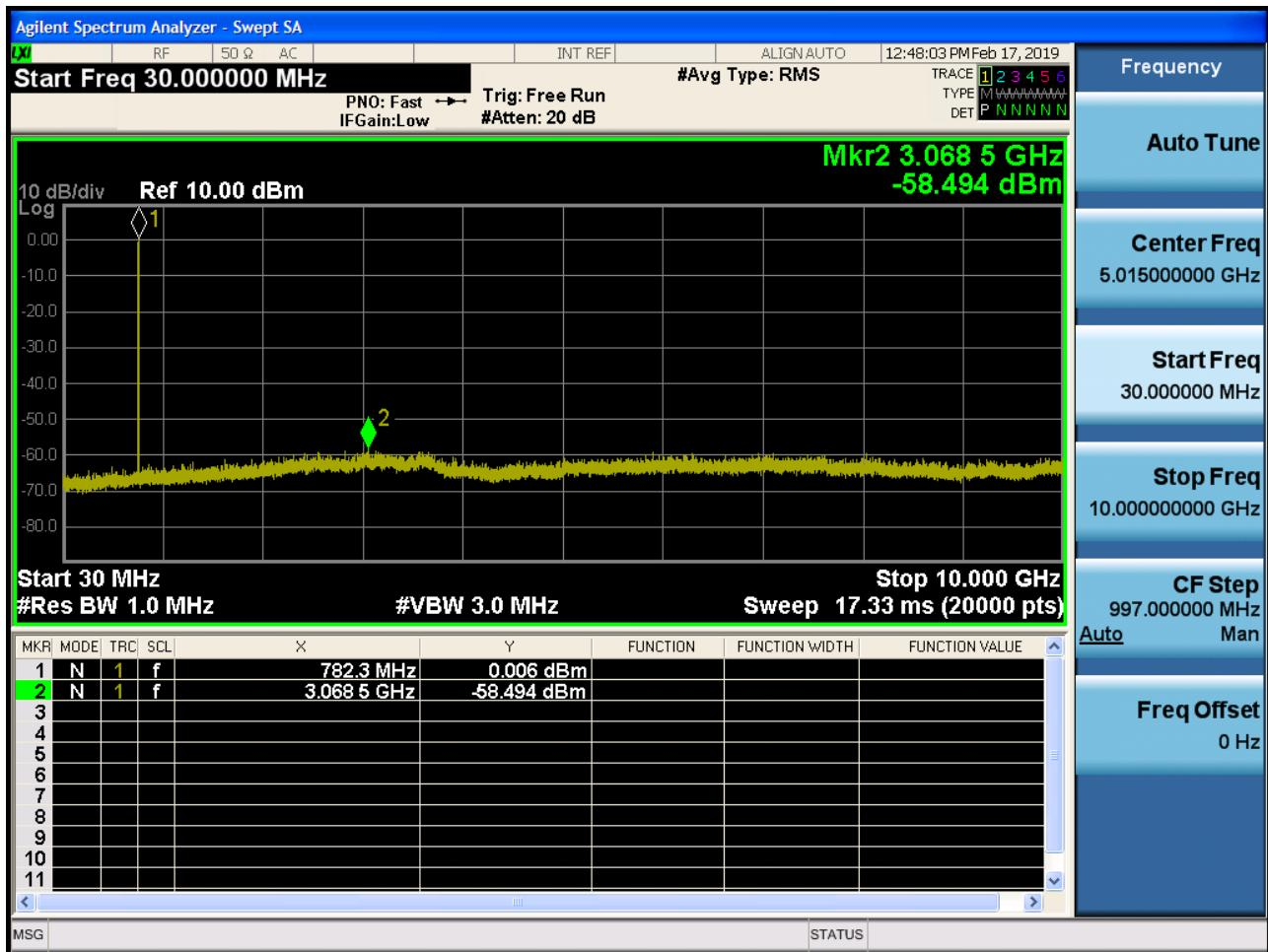
BAND 13. Conducted Spurious Plot (Ch.23230 10 MHz QPSK)
