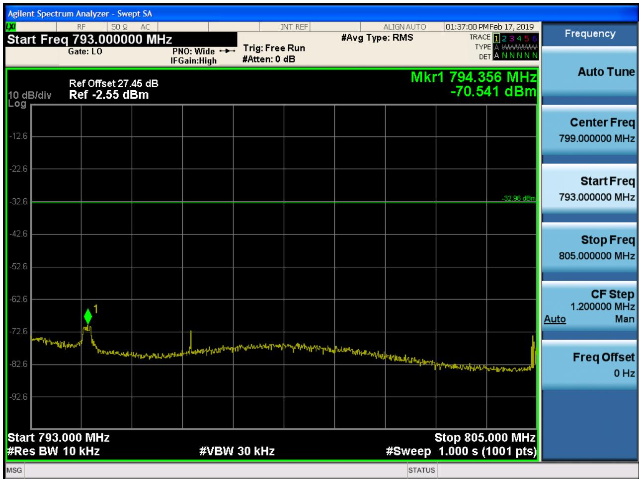
Band 13 Upper Emission Mask (793 MHz ~805 MHz) Plot (5M BW Ch.23255 QPSK\_Full RB)
