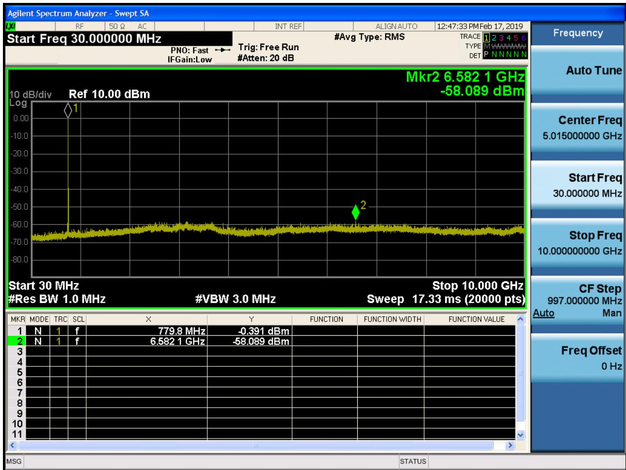
BAND 13. Conducted Spurious Plot (23255ch\_5MHz\_QPSK)
