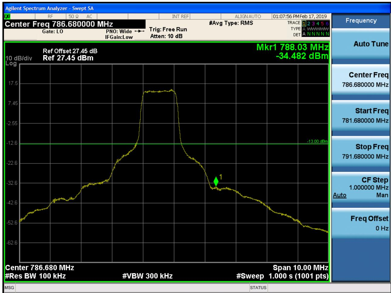
Band 13 Upper Emission Mask (793 MHz ~805 MHz) Plot (5M BW Ch.23255 QPSK\_1RB)
