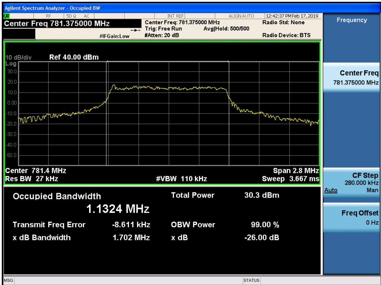
BAND 13. Occupied Bandwidth Plot (Ch.23230 QPSK) 10 MHz
