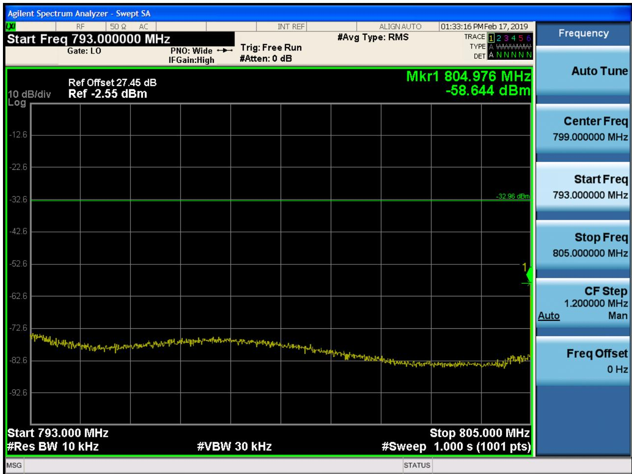
BAND 13. Conducted Spurious Plot (23205ch\_5MHz\_QPSK)
