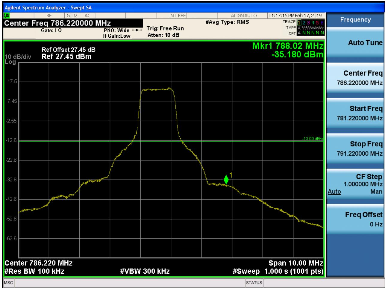
Band 13 Upper Emission Mask (793 MHz ~805 MHz) Plot (10M BW Ch.23230 QPSK\_1RB)
