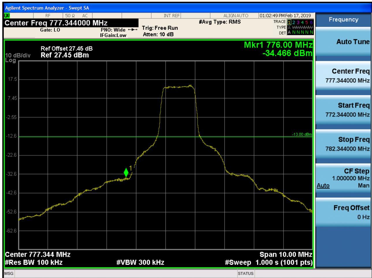
Band 13 Lower Emission Mask (763 MHz ~ 775 MHz) Plot (5M BW Ch.23205 QPSK\_1RB)
