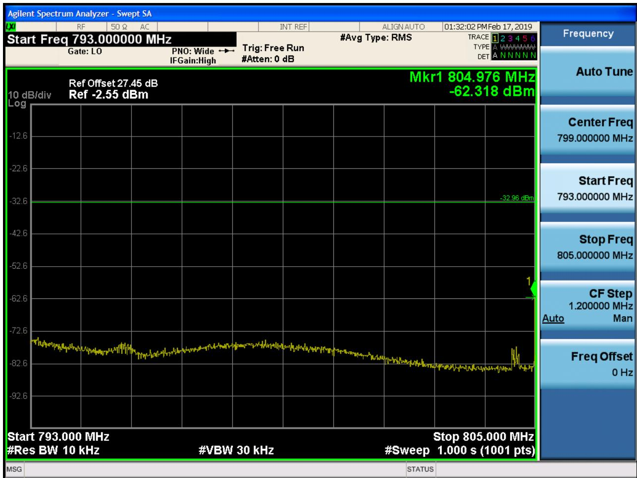
Band 13 Upper Emission Mask (793 MHz ~805 MHz) Plot (10M BW Ch.23230 QPSK\_Full RB)
