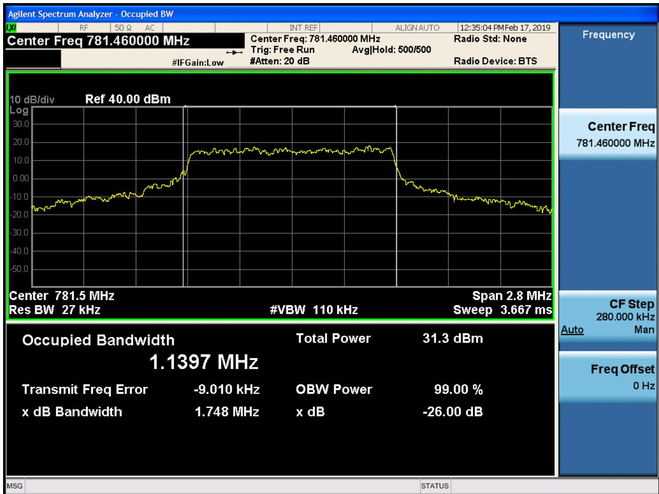
BAND 13. Occupied Bandwidth Plot (Ch.23230 16-QAM) 10 MHz
