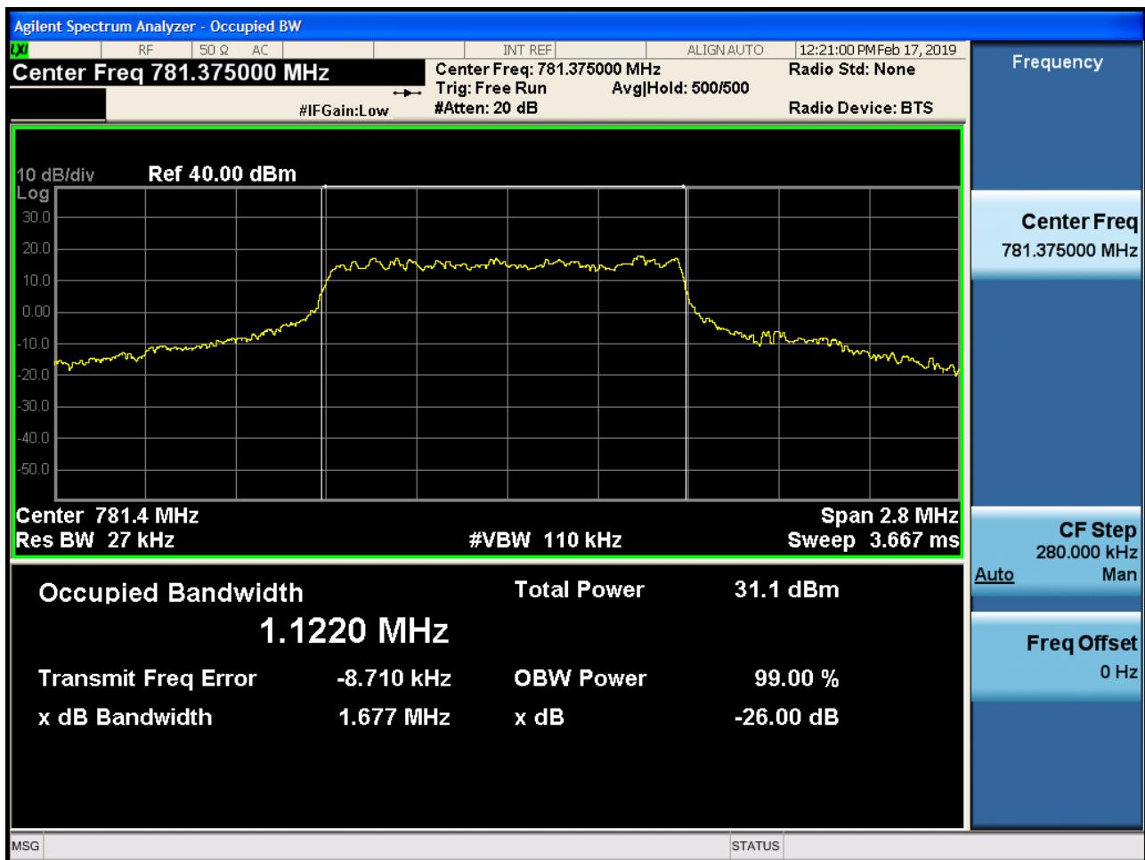
BAND 13. Occupied Bandwidth Plot (Ch.23230 16-QAM) 5 MHz
