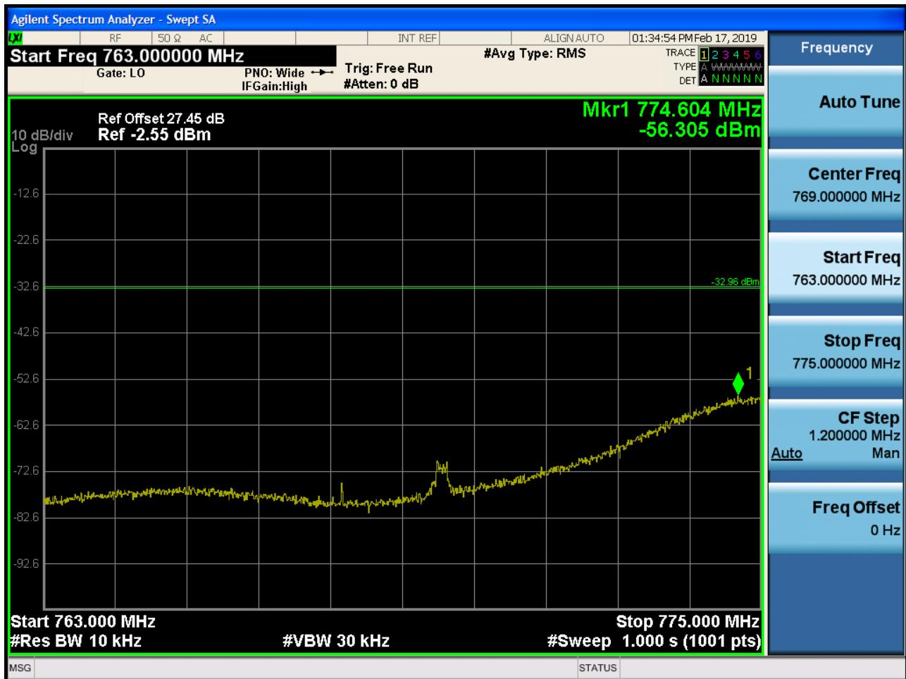
Band 13 Lower Emission Mask (763 MHz ~ 775 MHz) Plot (5M BW Ch.23205 QPSK\_Full RB)
