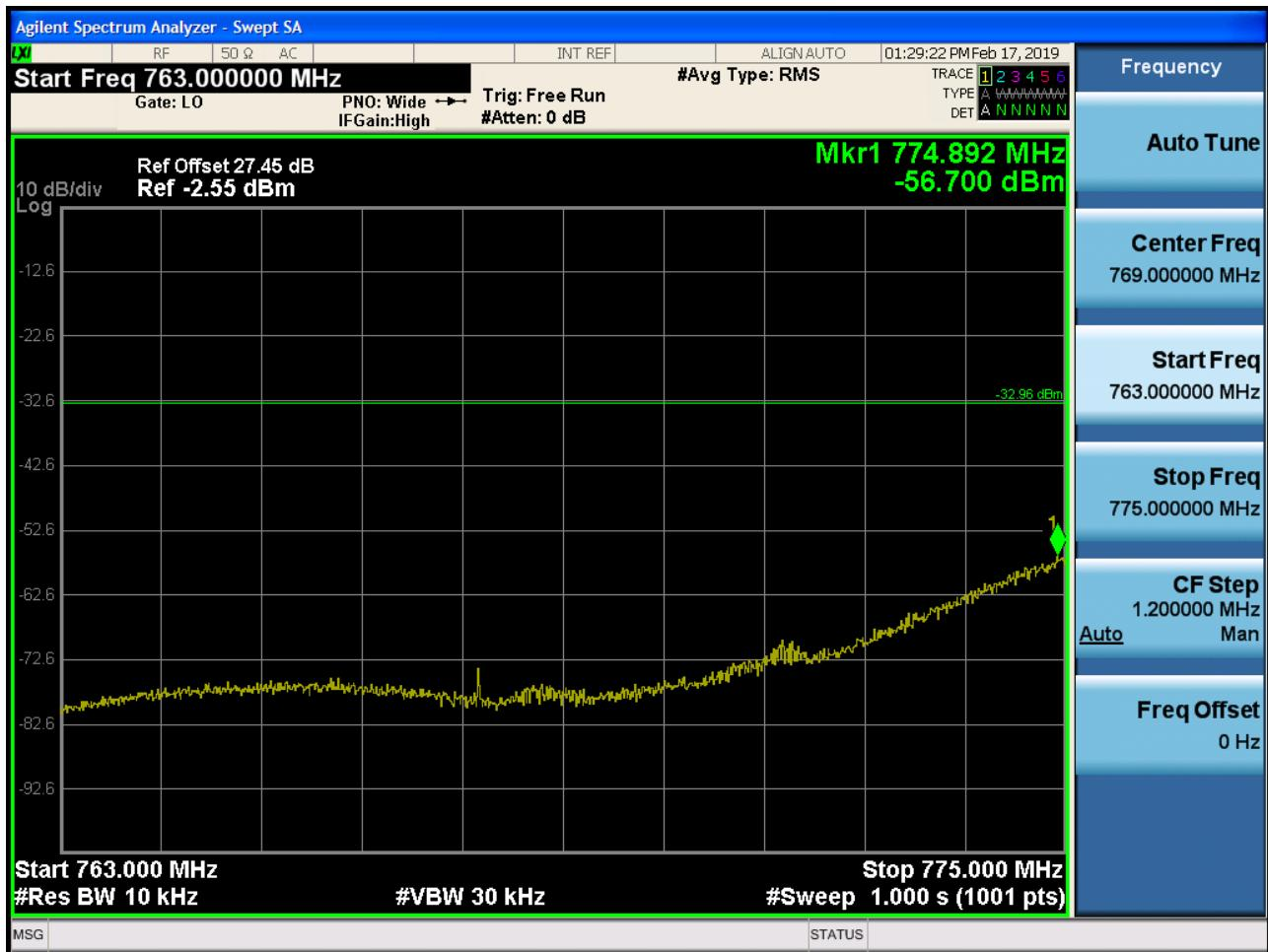
Band 13 Lower Emission Mask (763 MHz ~ 775 MHz) Plot (10M BW Ch.23230 QPSK\_Full RB)
