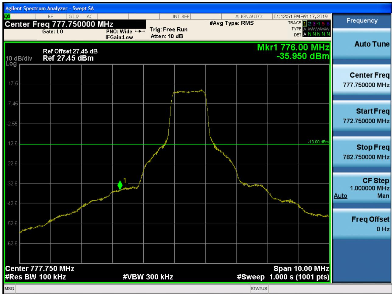
Band 13 Lower Emission Mask (763 MHz ~ 775 MHz) Plot (10M BW Ch.23230 QPSK\_1RB)
