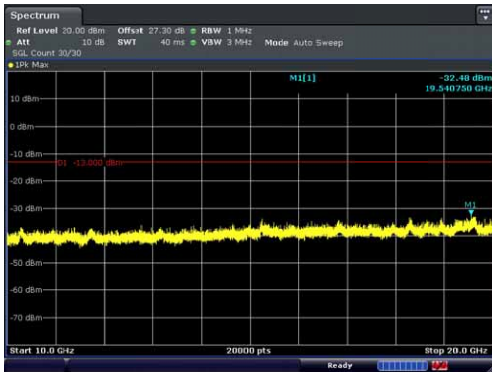
BAND 25. Conducted Spurious Plot_2 (26047ch_1.4MHz_QPSK_RB 1_0)
