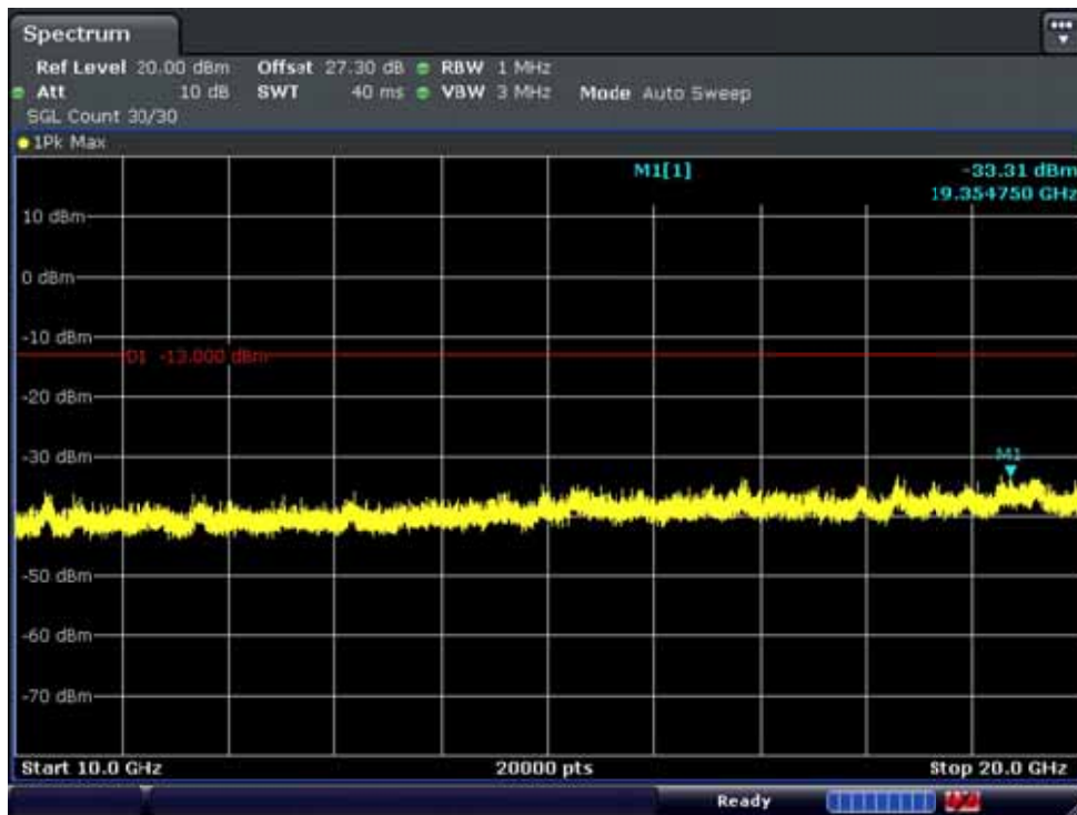
BAND 25. Conducted Spurious Plot_2 (26140ch_20MHz_QPSK_RB 1_0)
