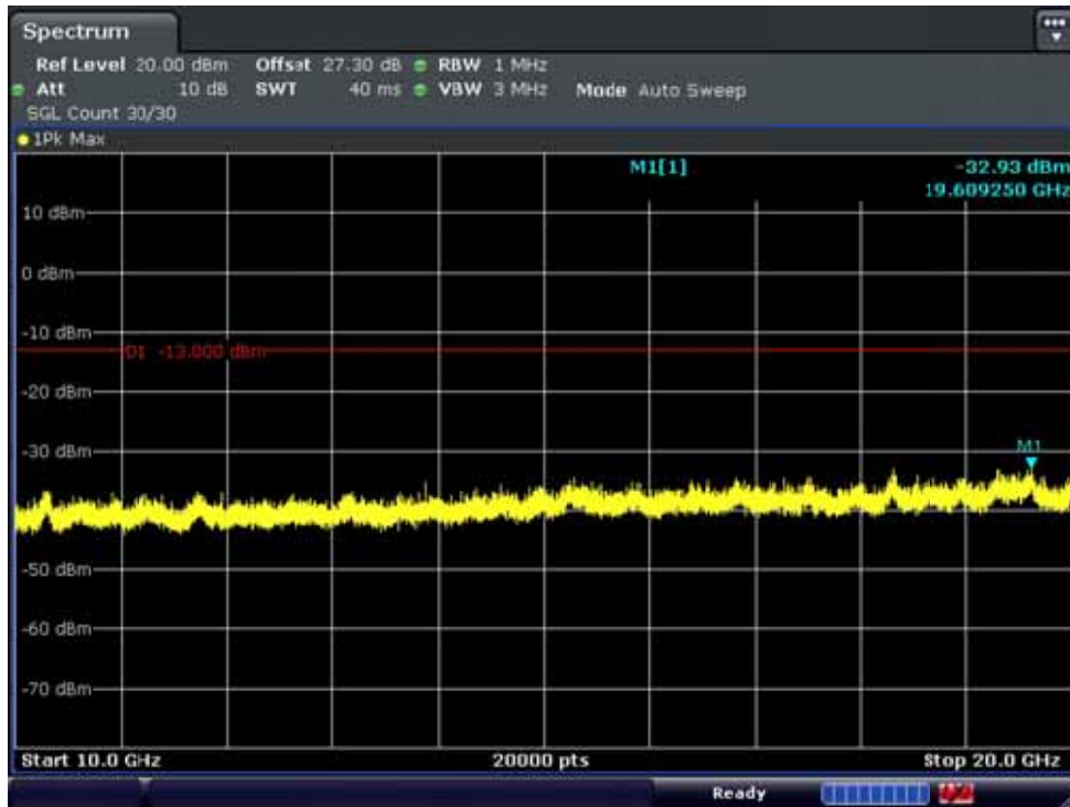
BAND 25. Conducted Spurious Plot_2 (26115ch_15MHz_QPSK_RB 1_0)
