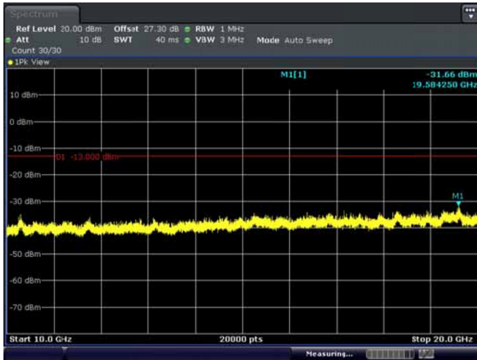
BAND 25. Conducted Spurious Plot_2 (26090ch_10MHz_QPSK_RB 1_0)
