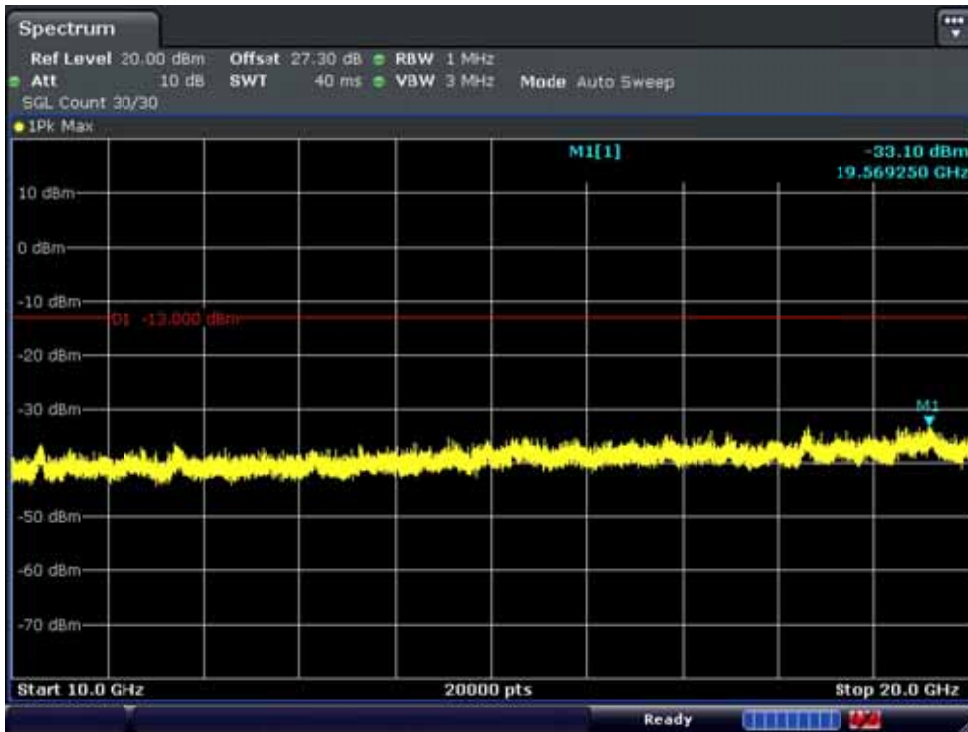
BAND 25. Conducted Spurious Plot_2 (26365ch_1.4MHz_QPSK_RB 1_0)
