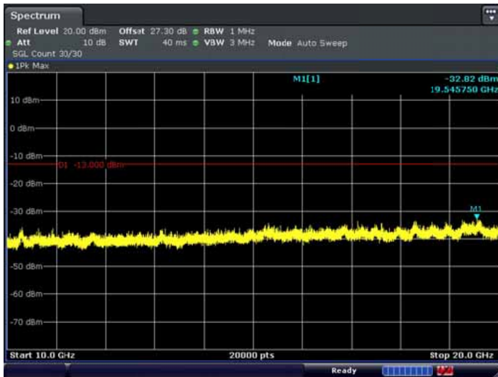
BAND 25. Conducted Spurious Plot_2 (26365ch_15MHz_QPSK_RB 1_0)
