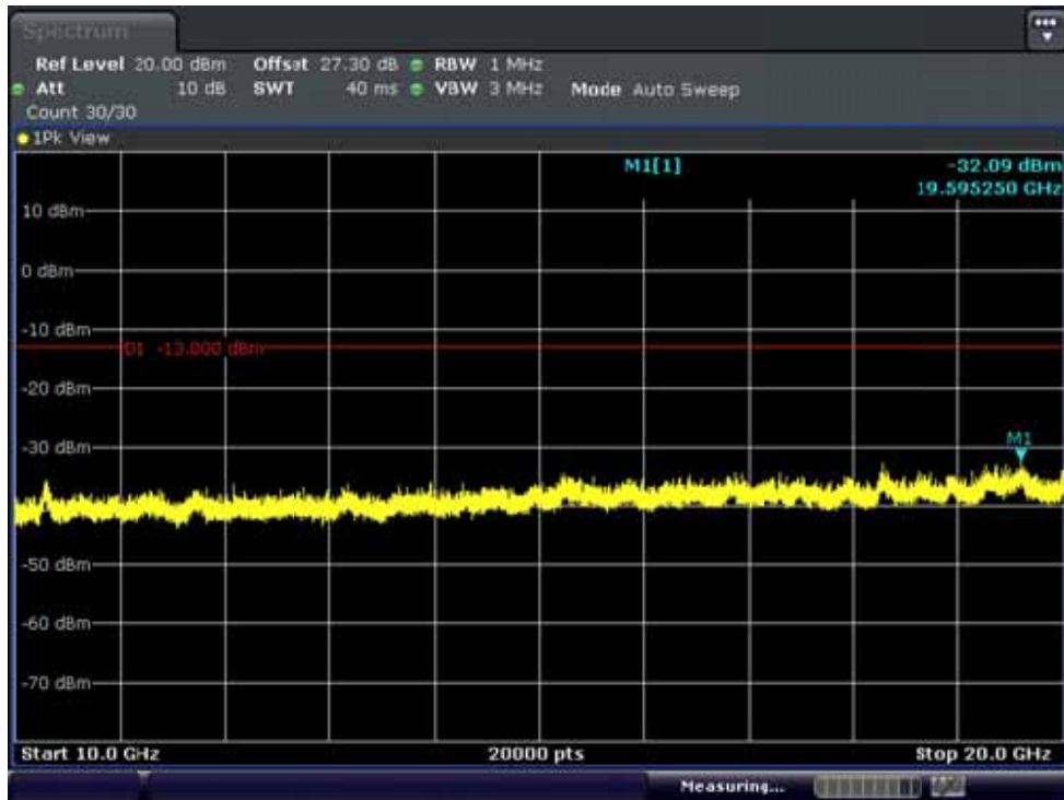
BAND 25. Conducted Spurious Plot_2 (26365ch_10MHz_QPSK_RB 1_0)
