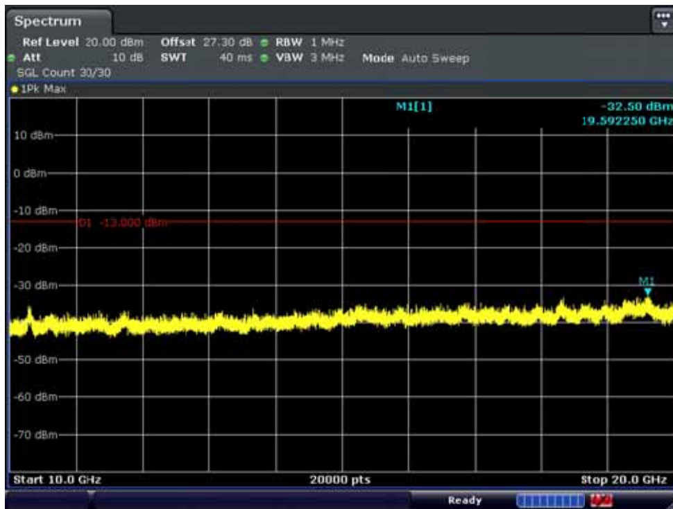
BAND 25 . Conducted Spurious Plot_2 (26665ch_5MHz_QPSK_RB 1_0)
