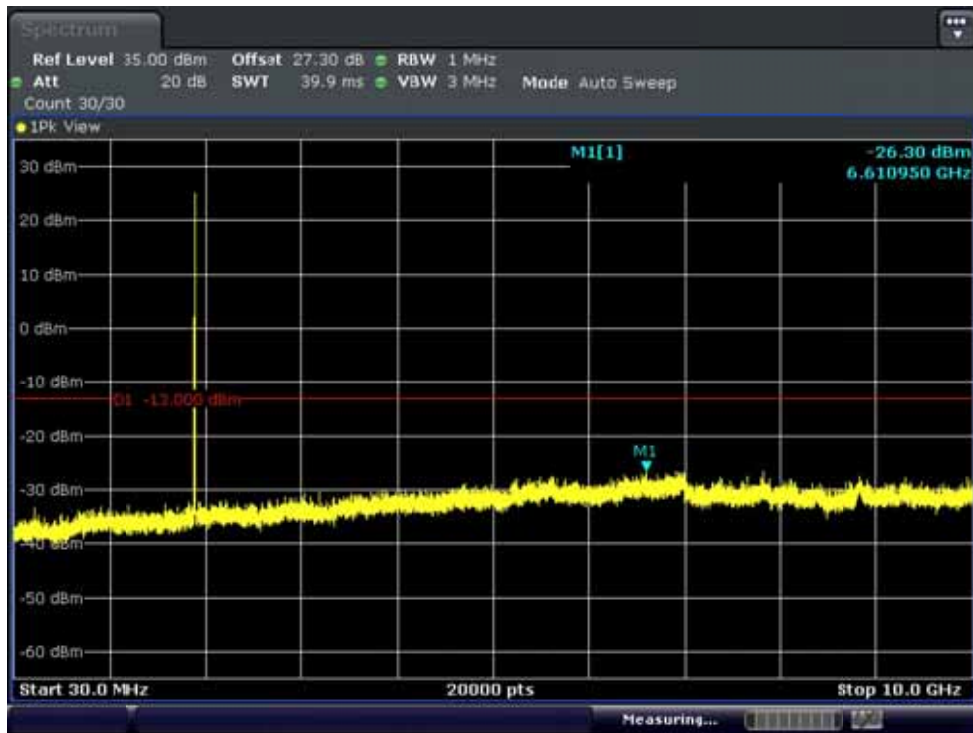
BAND 25. Conducted Spurious Plot_1 (26640ch_10MHz_QPSK_RB 1_0)
