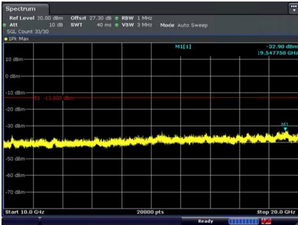
BAND 25. Conducted Spurious Plot_2 (26065ch_5MHz_QPSK_RB 1_0)
