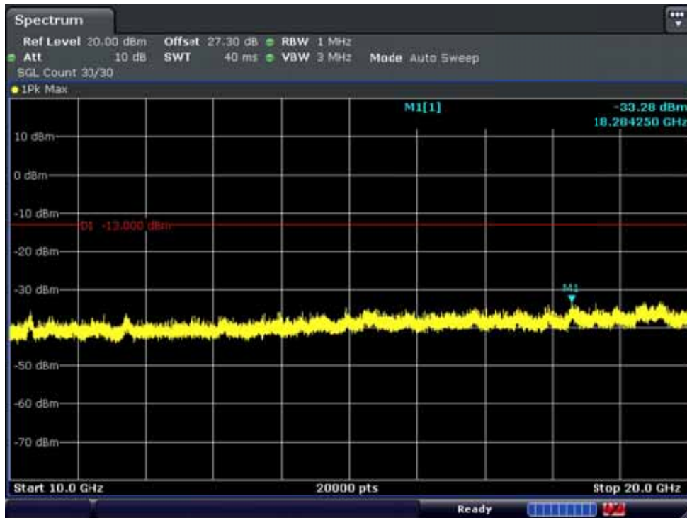
BAND 25 . Conducted Spurious Plot_2 (26683ch_1.4MHz_QPSK_RB 1_0)
