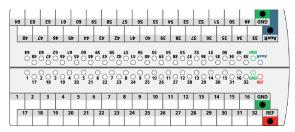
Figure 2: 64 channel electrode label.
