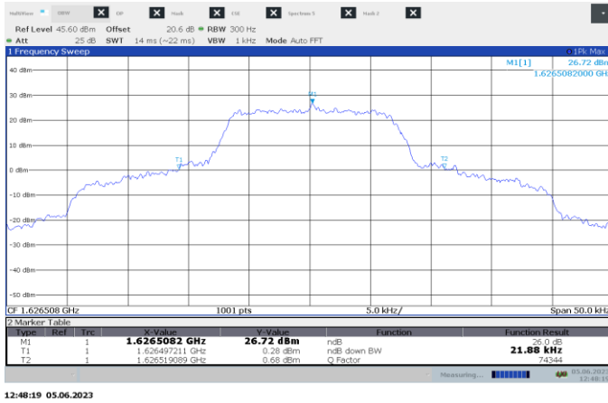
Figure 7.1-28: 26 dB bandwidth on low channel – Waveform Z
