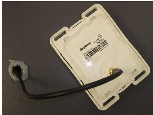
Figure 29 Apply Silicone to Hole in Asset
