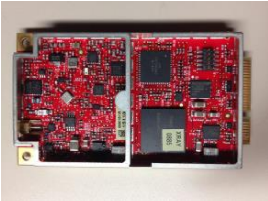
Figure 4.1 OGi Modem Internal Photo –Top view
