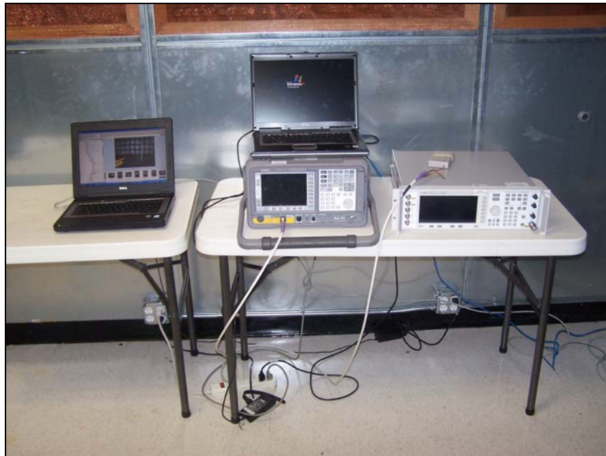
Photograph 7. Peak Power Spectral Density, Test Setup
