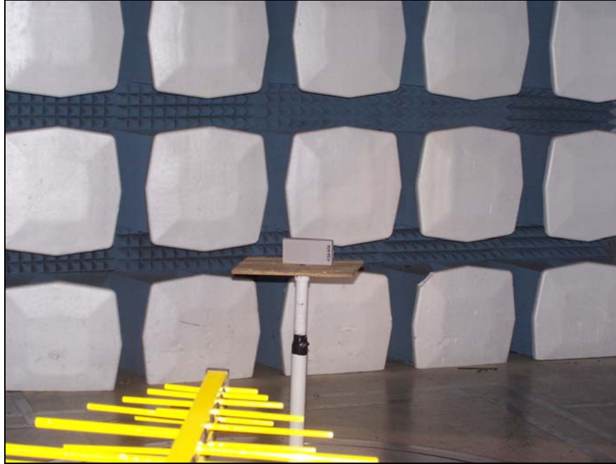
Photograph 2. Radiated Emission Test Setup 30 MHz - 1 GHz
