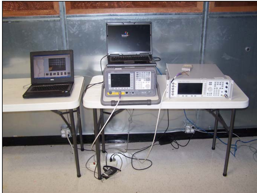
Photograph 6. Spurious Conducted Emissions, Test Setup
