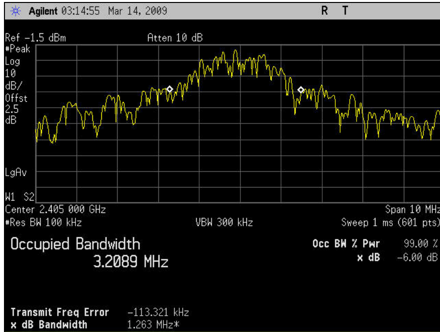
Plot 3. 6 dB Occupied Bandwidth, Low Channel
