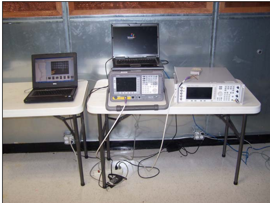
Photograph 7. Peak Power Spectral Density, Test Setup
