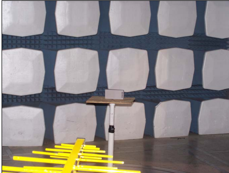
Photograph 2. Radiated Emission Test Setup 30 MHz - 1 GHz
