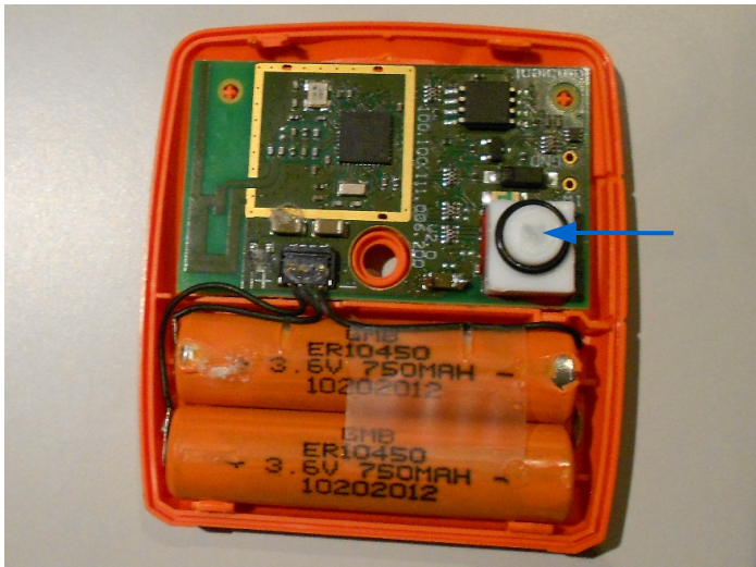
PCB front-side SP3000TH, placement of humidity sensor:
