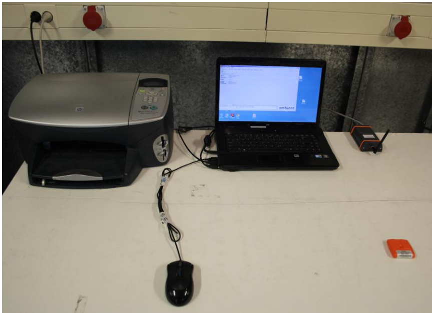
Photo 6b: Set-up for AC Power Line Conducted Emissions, EUT with Serial to USB connection
