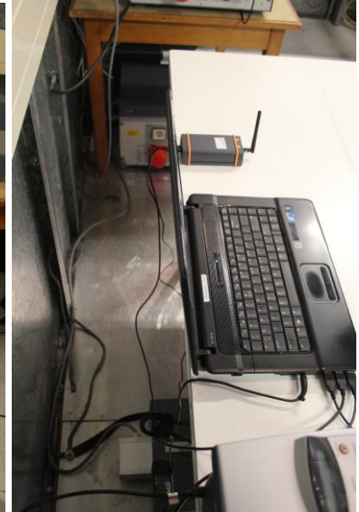
Photo 5a: Set-up for AC Power Line Conducted Emissions, EUT with USB connection
