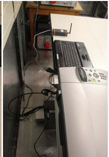
Photo 6b: Set-up for AC Power Line Conducted Emissions, EUT with Serial to USB connection
