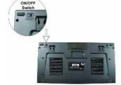
Power the keyboard switching it "ON". The switch is found at the back of the keyboard.
