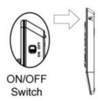
Power the keyboard switching it "ON". The power switch is found on the night edge of the keyboard.
