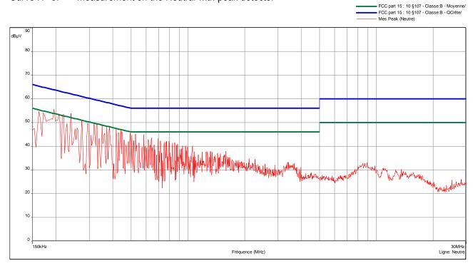
Curve N° 6: measurement on the Line with peak detector
