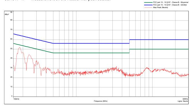
Curve N° 2: measurement on the Line with peak detector
