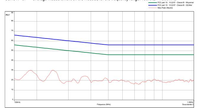
Curve N° 4: average measurement on the Line, for the frequency range: 150KHz – 1.500MHz
