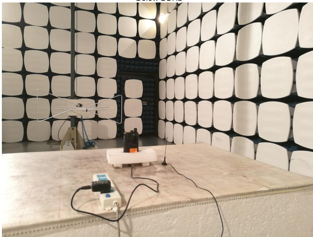
Radiated Spurious Emission Below 1GHz
