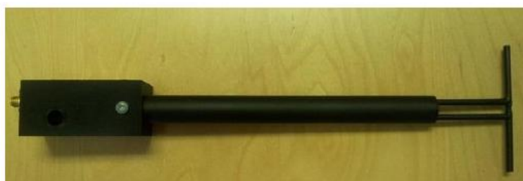
Figure 1 – MVG COMOSAR Validation Dipole
