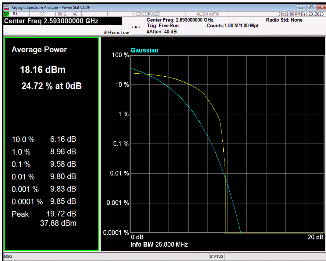
Band41 QPSK BW=15MHz Channel=40620 RB Size=1 Position=#0
