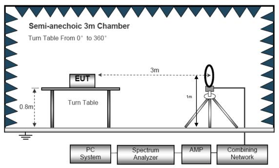
(B) Radiated Emission Test-Up Frequency 30MHz~1GHz
