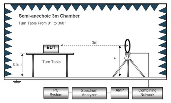
(B) Radiated Emission Test-Up Frequency 30MHz~1GHz
