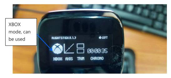
5. 3 If the OLED is displayed in PC state as shown below, you need to switch to XBOX mode to
