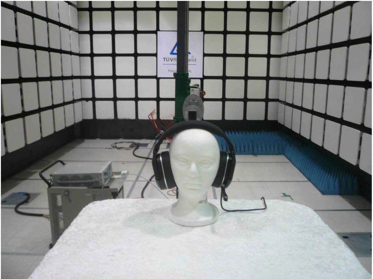
Figure 7: Test Setup for 18 GHz to 26 GHz (Front View)
