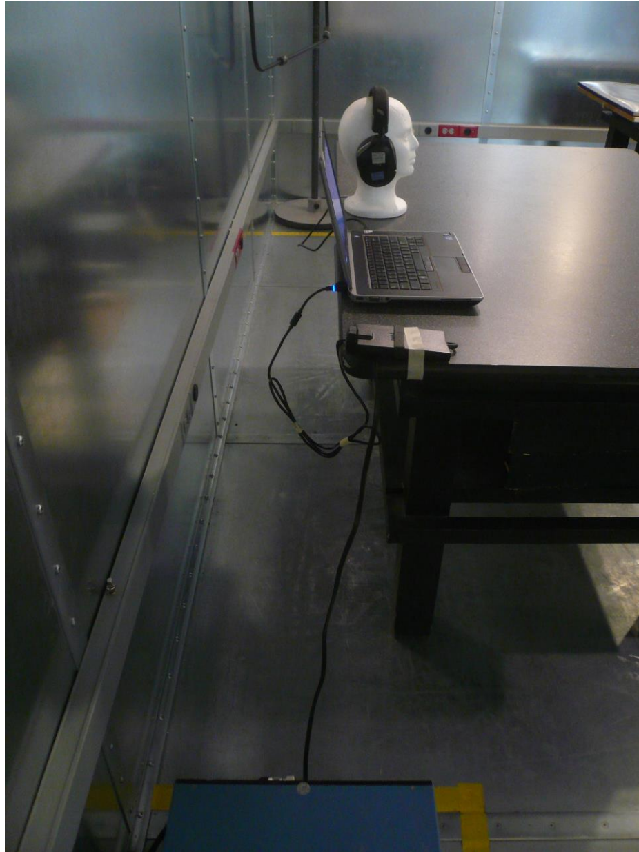
Figure 11: AC Conducted Emission Test Setup (Rear View)
