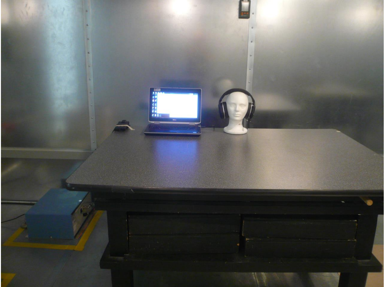
Figure 10: AC Conducted Emission Test Setup (Front View)
