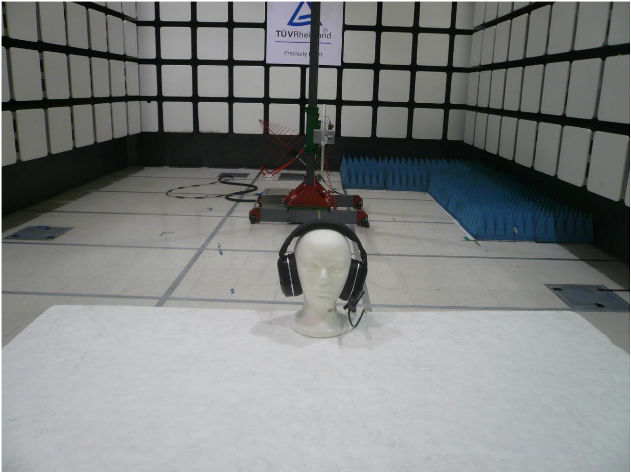
Figure 1: Test Setup for 9 kHz to 30 MHz (Front View)
